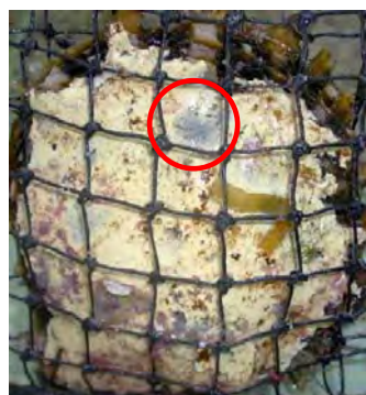
Figure 15.4. SF coated shell after 8 months (a bivalve scar is highlighted by the circle).
