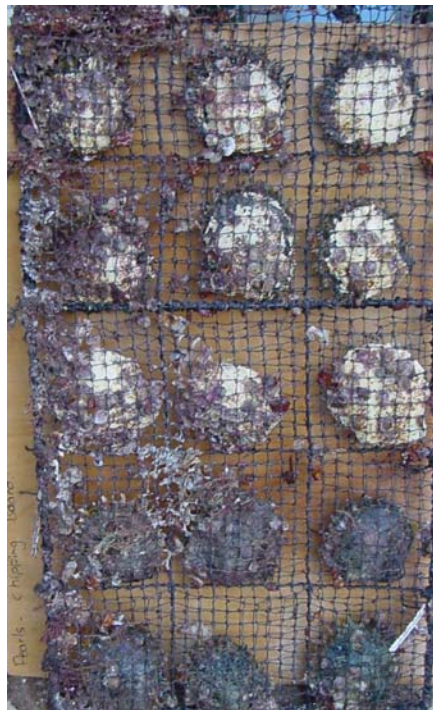
Figure 15.2. Panel with shell, after washing with high pressure water at 16 weeks. SF coated shell are in the top three rows and controls in the bottom two rows. Bivalve fouling can be seen on coated shell.
