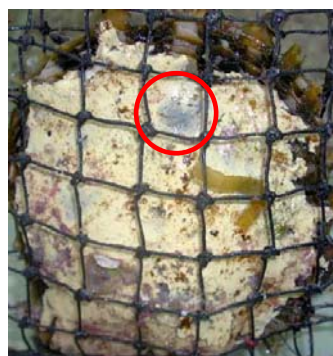
Figure 15.4. SF coated shell after 8 months (a bivalve scar is highlighted by the circle).
