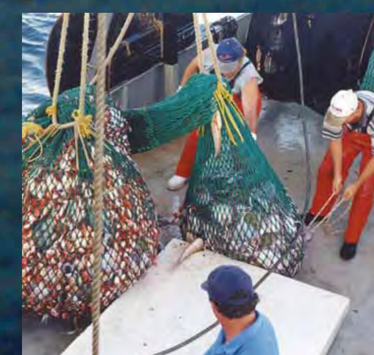
Testing a modified codend using the trouser trawl
