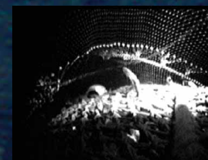
Underwater image of fish escaping from a codend
