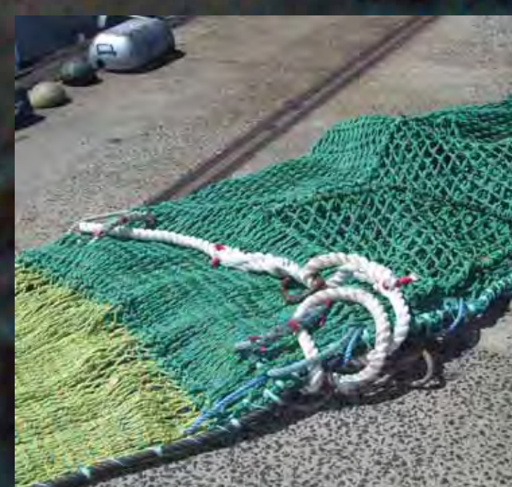
A codend with a Square mesh panel being readied for sea
