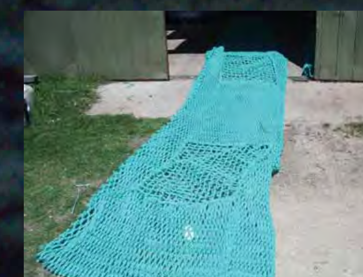
Smaller, strategically positioned square mesh windows in a codend under construction
