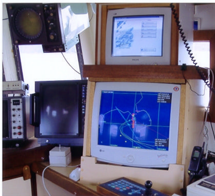
Figure 1. OLRAC software (upper) running in conjunction with C-plot on dual monitors installed on the Huon Petrel during E-boat trials.
