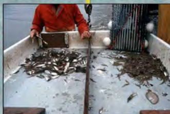
The Nordmore-grid has reduced the bycatch from estuarine trawlers by up to 90% with no loss in prawn catches.
