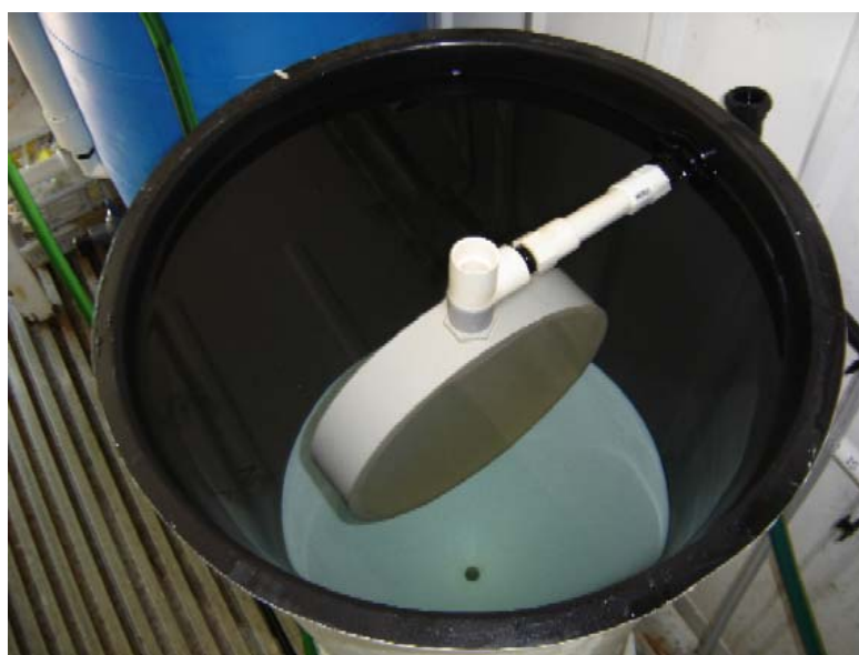
Fig 7. Banjo screen fitted to the over flow of a larval rearing vessel (note the conical bottom of the vessel).
