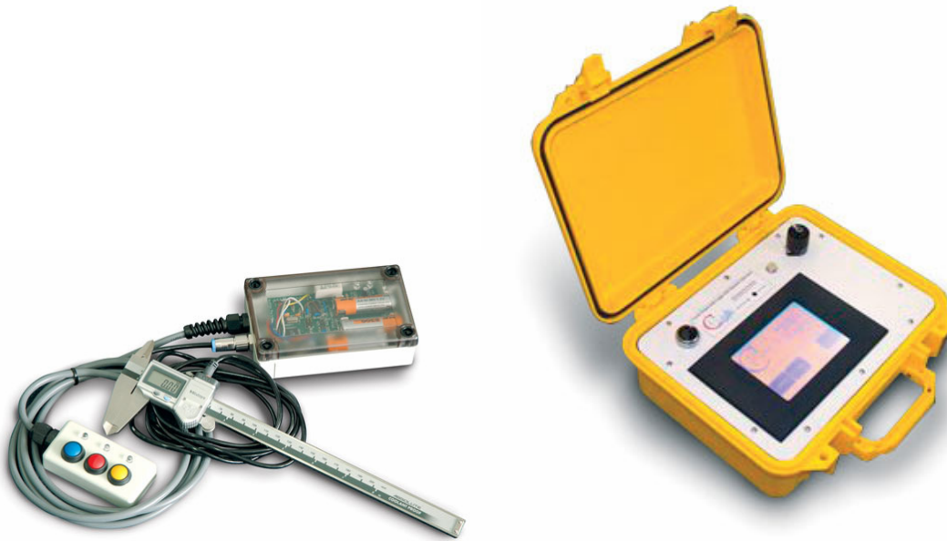
Figure 12. Electronic options developed for recording length measurements from callipers. The waterproof vernier calliper logbook (left) stores gender, berried state, length and units, date, time. The touch screen logbook (right) can be connected to electronic callipers and easily programmed to store more extensive data, such as tag number, damage (missing limbs), individual pot ID, and bycatch. The basic calliper logbook has been deployed with several fishers and now serves as the main system for obtaining size-structure data for the crab fishery.
