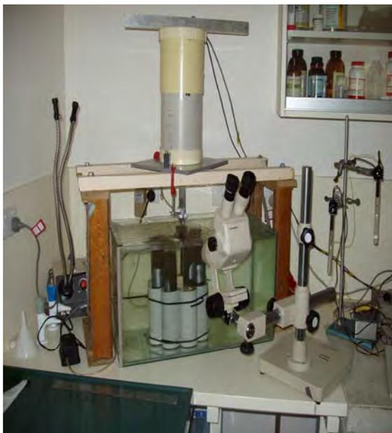
**Figure 2. Experimental set-up for measurement of oxygen penetration depths.**
