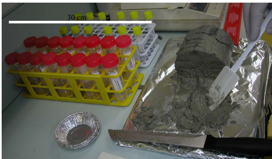
Figure 7.5. Extrusion of the sediment core and transfer of homogenised sediment to centrifuge tubes.
