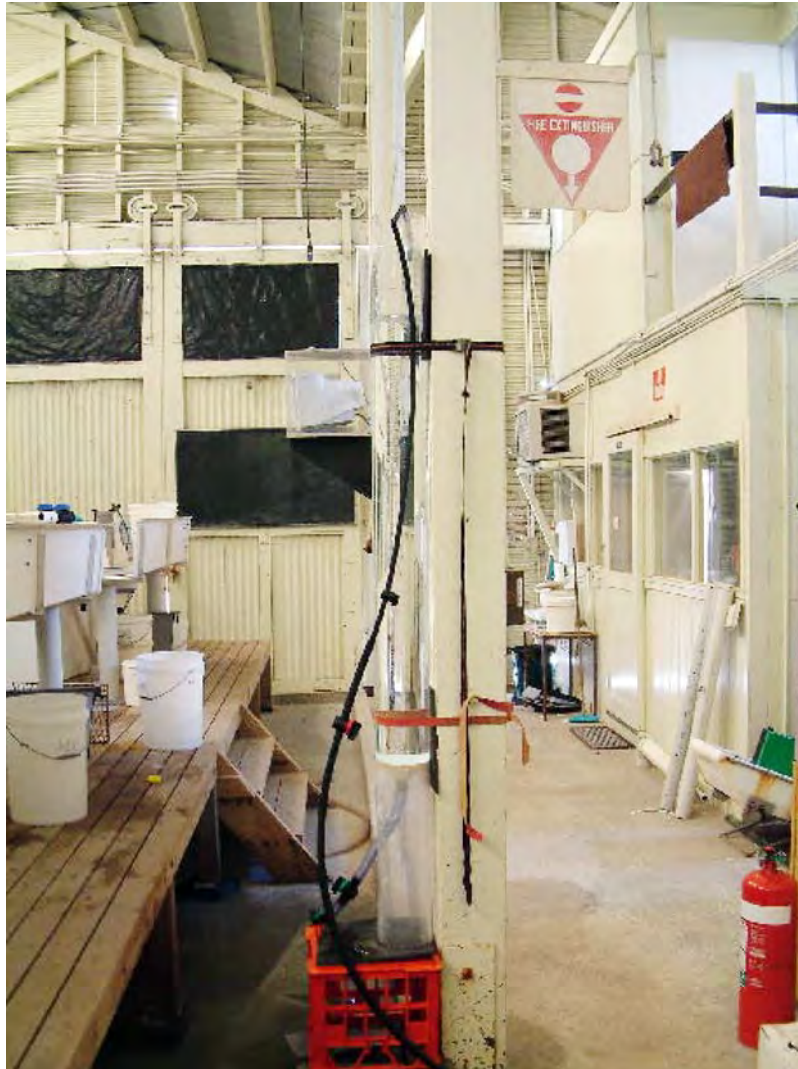
Photo 1. Experimental test vessel, a 2 m tall, 145 mm in diameter cylinder used to determine the sinking rates of 11 commercially available microdiets.
