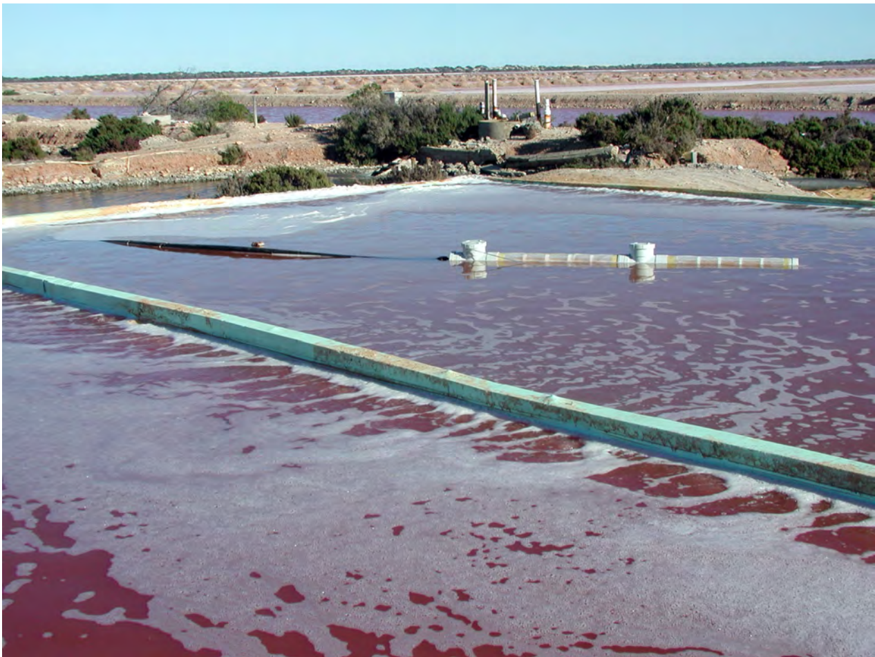
Figure 3. First stage filter in pond to remove cysts and nauplii.
