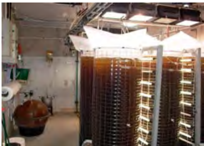
Figure 10. Continuous microalgal production system (10 x 400L bags) at SAASC.
