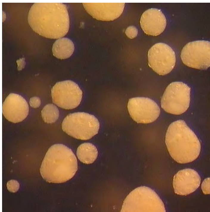
Figure 1. Photomicrograph showing the appearance of food microparticles prepared by internal gelation.
