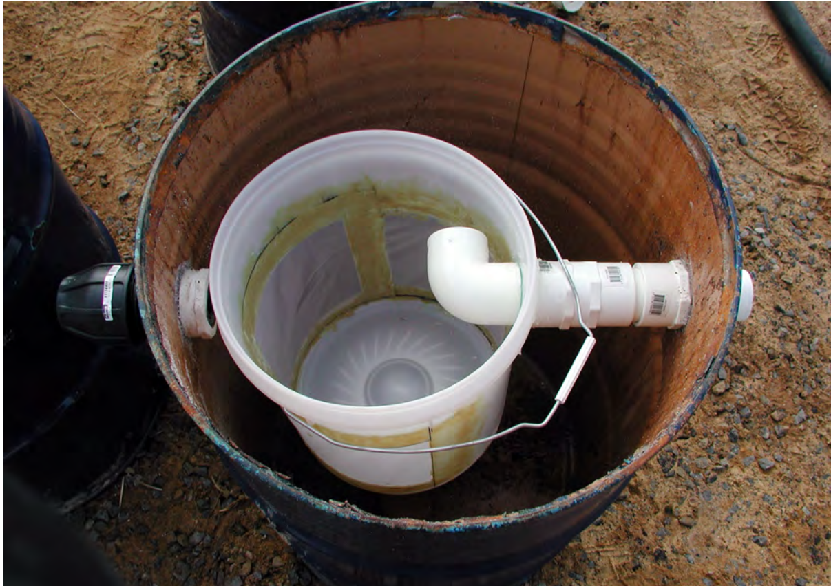
Figure 6. Third stage filter to retain cysts.
