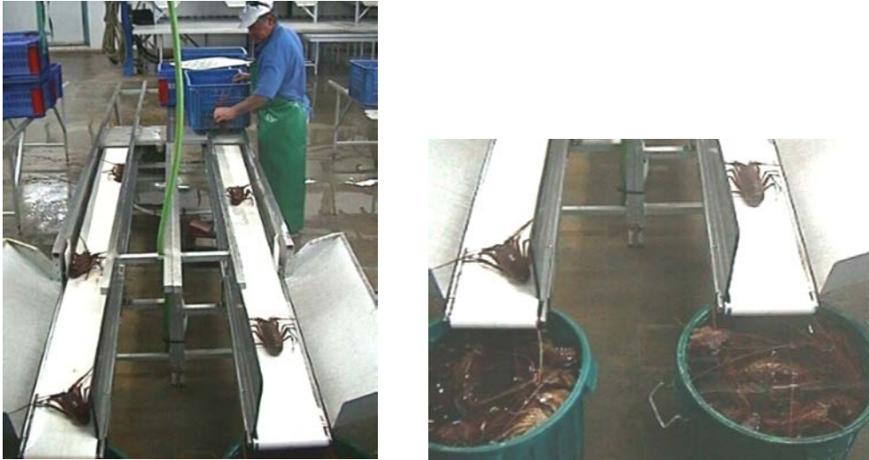
Figure 3) The set up used for investigating leg loss during freshwater drowning of red A-grade western rock lobsters. Lobsters were transported by conveyors to drowning tubs (right).
