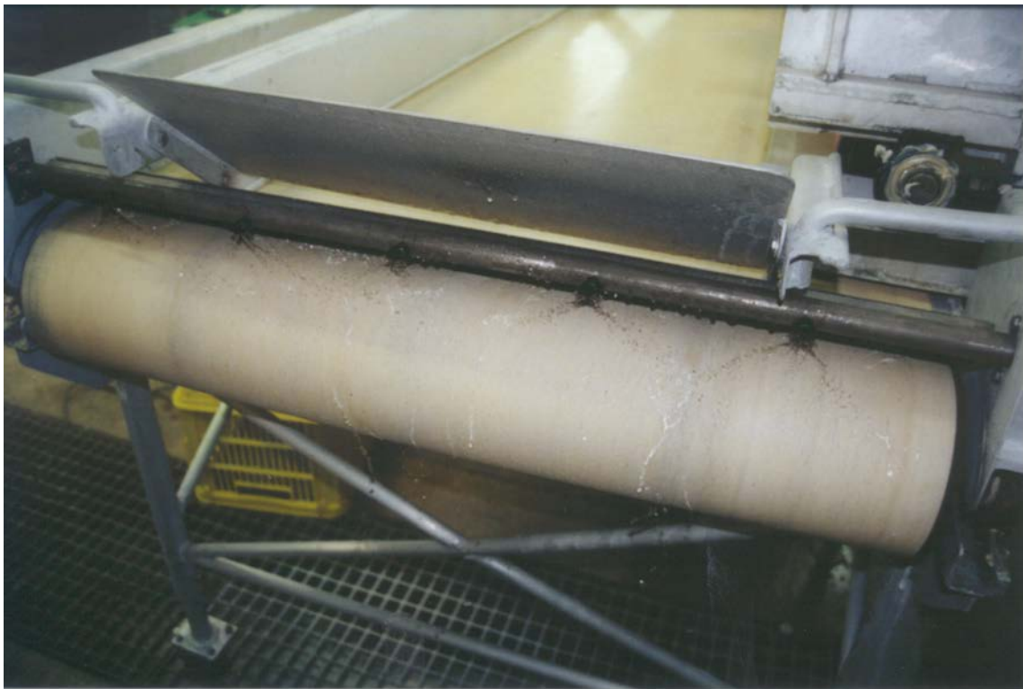
Figure 13) Processors have taken steps to reduce salt build up in factories. This figure shows freshwater sprays fitted to a belt used to convey lobsters past graders. The sprays continually wash the belt preventing salt build up.
