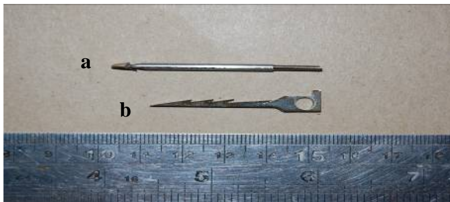
Figure 2. Lancets used to collect tissue simultaneously with the placement of conventional tags: (a) Cut and ground from stainless steel wire, 5 cm long (b) Laser-cut from sheet stainless steel, 4 cm long
