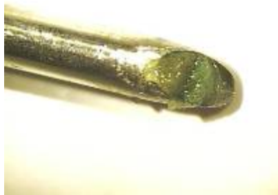
Figure 7. Hook-tip Sc272 showing a large amount of tissue with green colour that could have been a result of copper contamination
