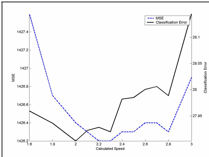
Figure 7.17 Error measures for various upper cut-off trawl speeds (m/s) in the EKP trawl signature
