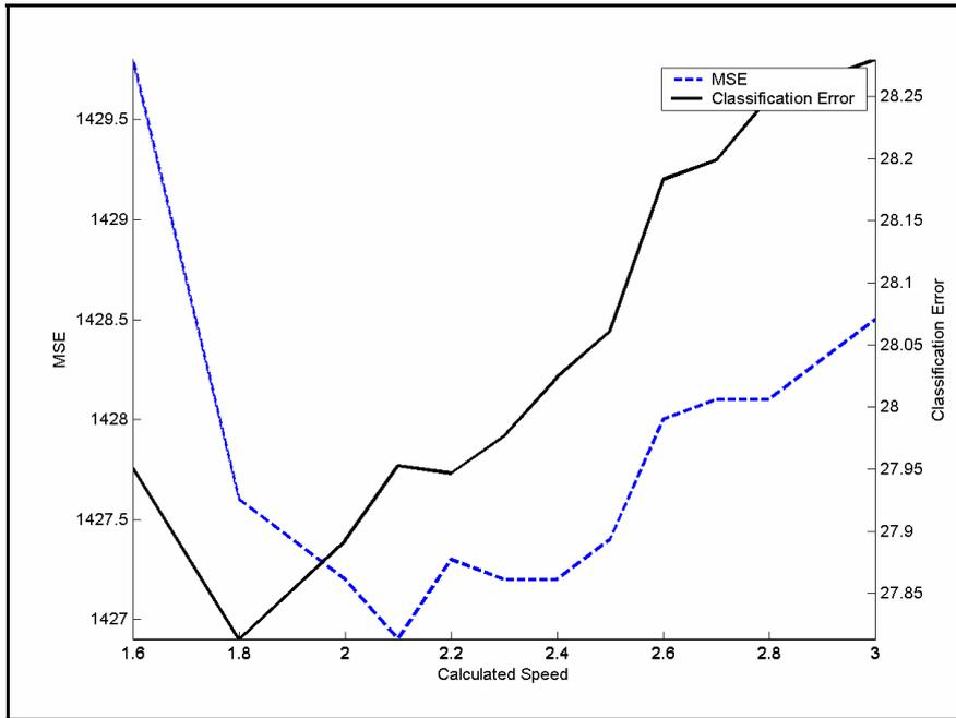
Figure 7.18 Error measures for various upper cut-off trawl speeds (m/s) in the tiger/endeavour prawns trawl signature
