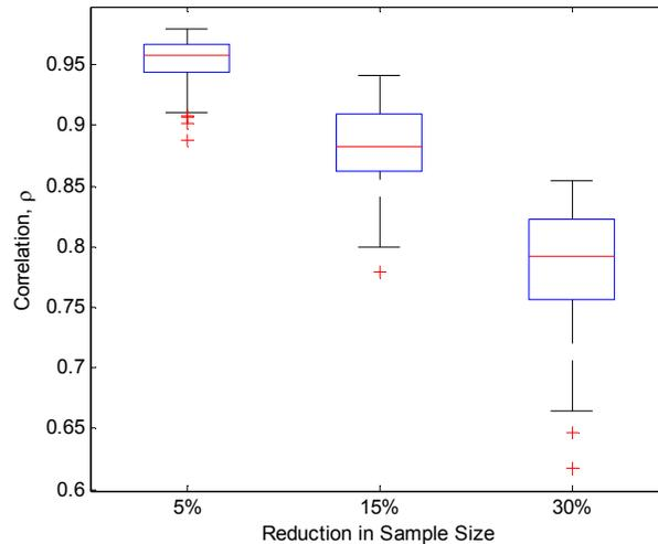
Figure 9.2. Box and whisker plots of correlations of original MaxEnt reconstruction and reconstructions with 5, 15 and 30% of random tows removed, both based on 100 Jackknife sample reconstructions. Data are for a one-week period in December 2003 in the shallow-water EKP fishery and consists of 703 tows.
