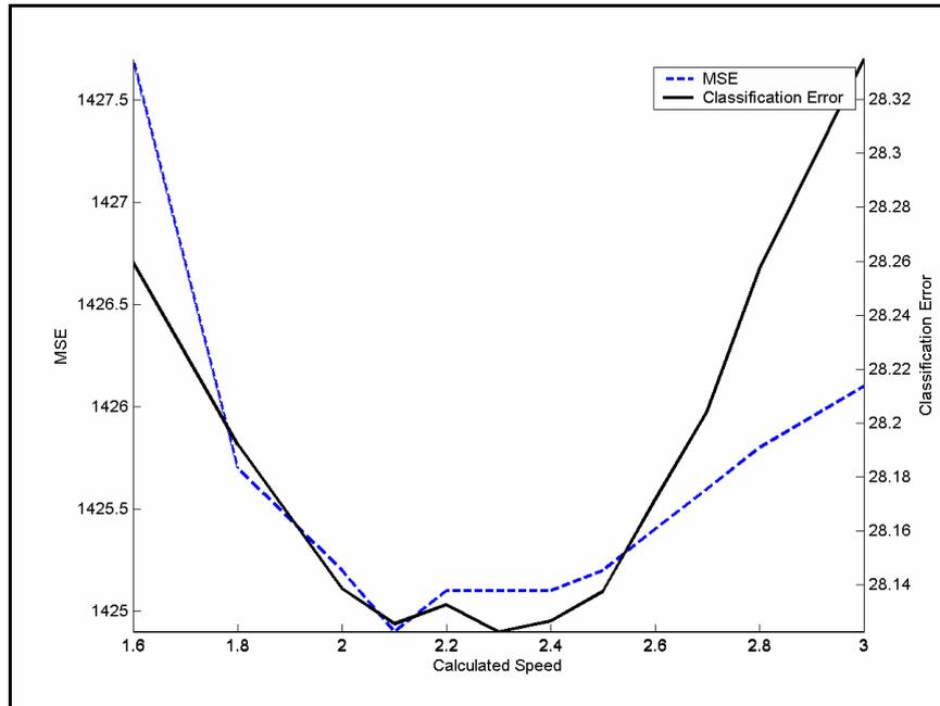
Figure 7.16 Error measures for various upper cut-off trawl speeds (m/s) in the scallop trawl signature
