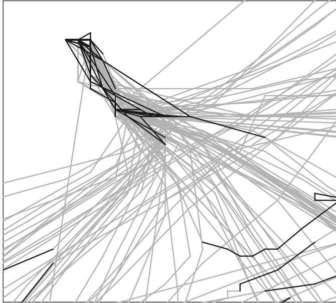
Figure 8.13 Plot of VMS data for a year in a particular region with HMM applied. Transects with trawl probability  $< 0.5$  denoted by grey lines and trawl probability  $\geq 0.5$  denoted by black.
