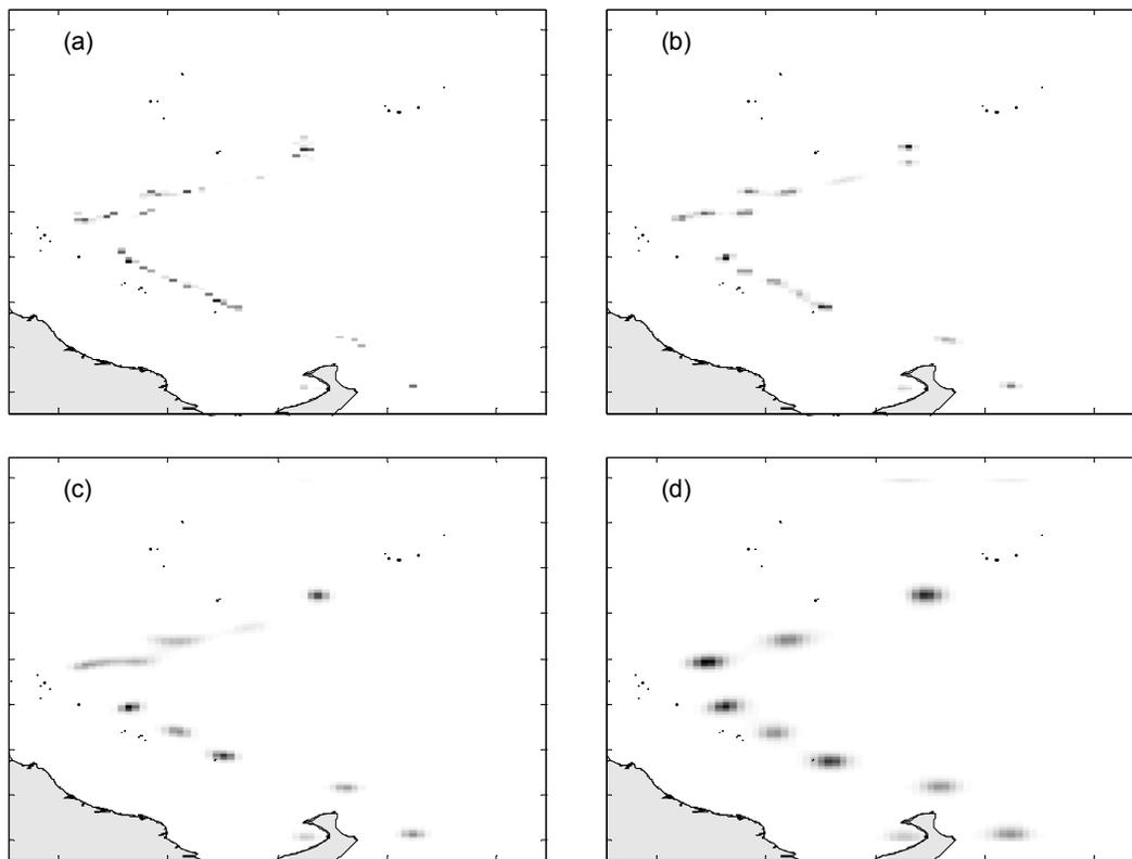
Figure 9.5. MaxEnt reconstructions of EKP distribution in the deepwater sector: (a) No ICF (b) ICF width of 3 (c) ICF width of 5 and (d) an ICF width of 8.
