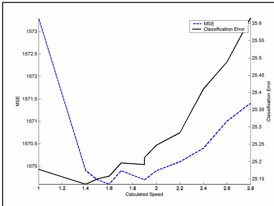
Figure 7.19 Error measures for various upper cut-off trawl speeds (m/s) in the banana prawn trawl signature
