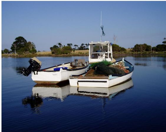
Haul seining in Gippsland Lakes. The seine is carried on the tender.
