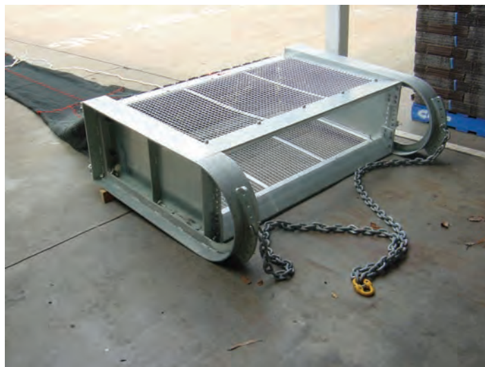
Figure 5.3-1: Epi-benthic sled used for sampling seabed fauna
