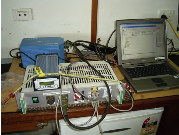
Figure 6.4-2: Set up with the Tracklink. The blue box is an Octans Gyrocompass, in the foreground is the interface rack which has inputs from gyrocompass, GPS (the Seastar is strapped to the top of the rack), the pitch and roll sensor and the heading sensor (gyrocompass). The laptop computer is running the Tracklink and storing data. The large black cable is the connection to the transceiver.
