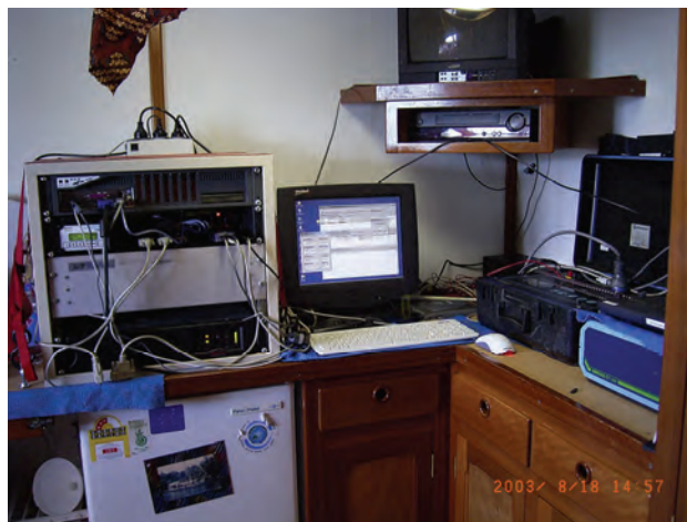
Figure 6.4-1: Setup on board ship with the LXT system. On the left is a rack with a UPS (black), the small box on the left above this is the Seastar (differential GPS) and above this to the right is a computer for data storage. On the right of the picture the blue box is the EY500 (echo-sounder) with the deck unit of the LXT to the left.
