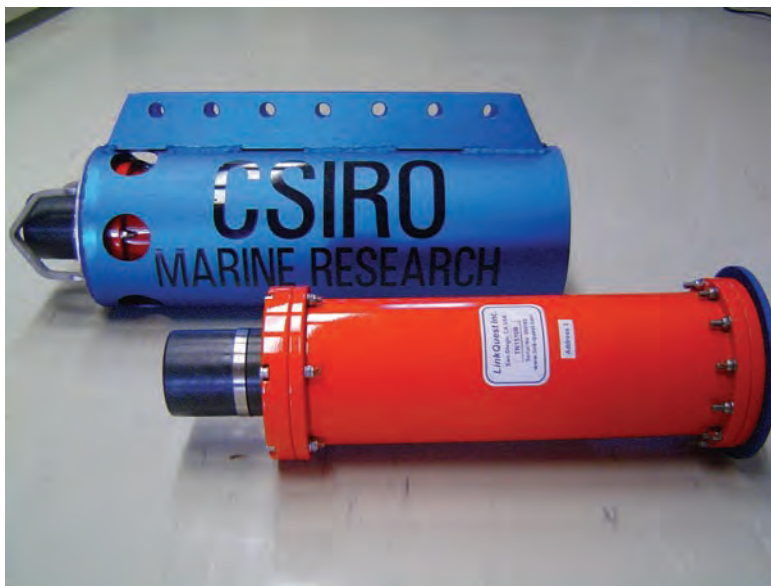
Figure 6.4-4: Foreground: Tracklink transponder. The transmitter/receiver antenna is in the black cylinder on the left end. The orange housing contains circuitry and batteries. Background: Transponder in protective housing.
