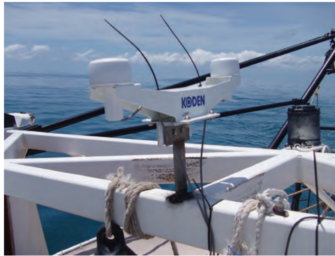
Figure 6.4-6: Koden GPS compass in position on trawler. The GPS antennas are in the ends of the arms
