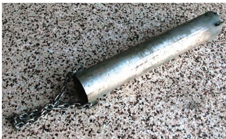
Figure 5.2-2: Pipe dredge used for sampling sediment. The dredge was towed from the chain bridle at the left. The pipe is sealed at the opposite end.
