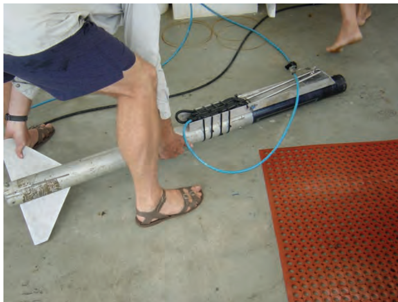
Figure 5.2-1: Side scan sonar used for surveying the experimental sites
