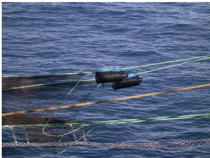
Figure 6.4-5: Transponders attached to trawl bridles between the trawl boards and the nets. The transponder housings have been wrapped in foam to provide further protection
