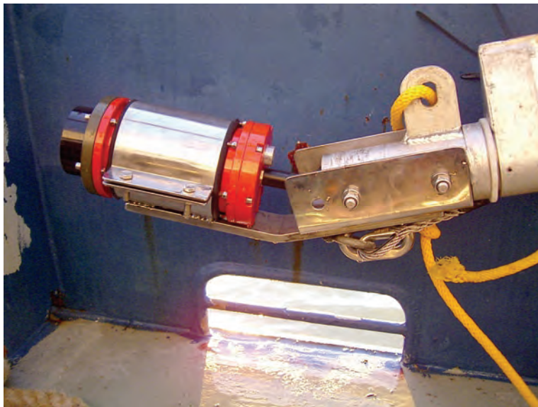
Figure 6.4-3: Transceiver mounted on end of pole that could be fixed to the side of the vessel
