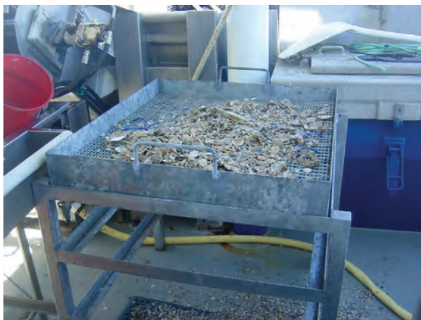
Figure 5.3-3: Mesh tray used for preliminary sorting of epi-benthic sled samples at sea.
