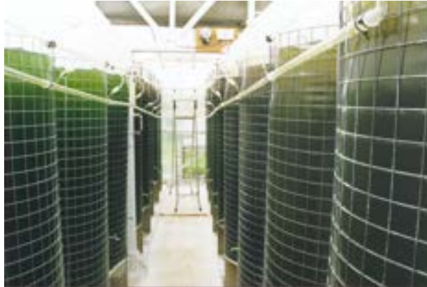
Semi-continuous algae bag system filled with pasteurised Seawater at the same rate as algae is harvested.
