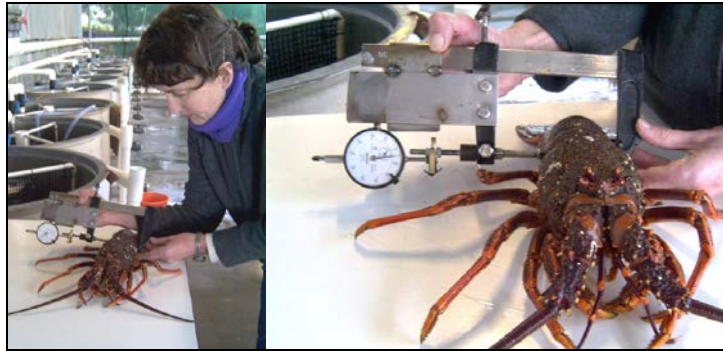
Figure 18. Prototype compression gauge being used to test shell compression across the tail (on the 2 nd abdominal segment).
