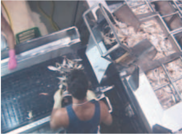
Catch transferred from hopper conveyor to sorting conveyor.
