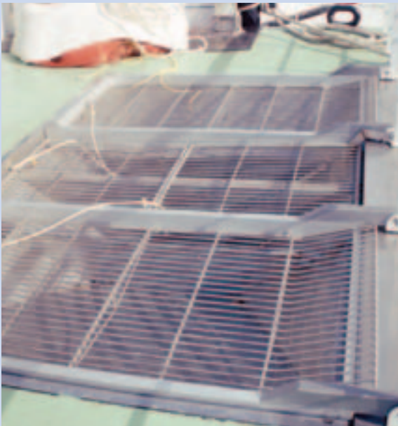
Grates (crab racks) on top deck. Catch is spilled onto grates and into the hopper below.
