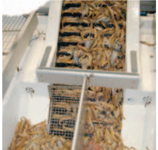
Prawns are removed from the hopper via a conveyor.
