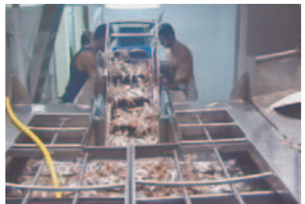
Catch held by flights on the belt of the hopper conveyor.
