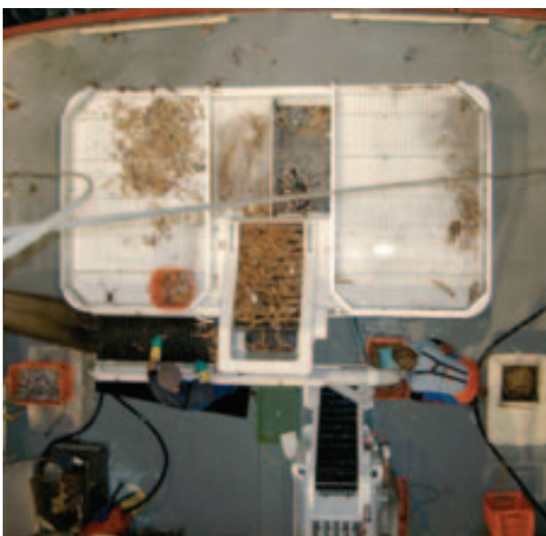
Hopper system with catch in hopper, crab racks, conveyors, discard chute and grader.
