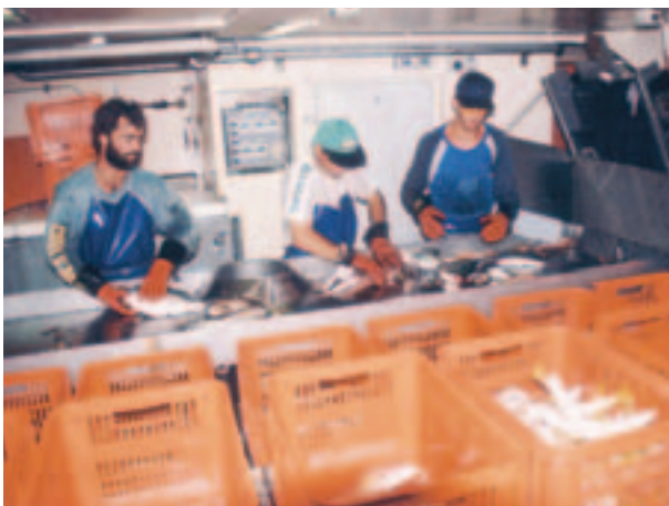
Fish sorting table with bycatch chute in the centre.
