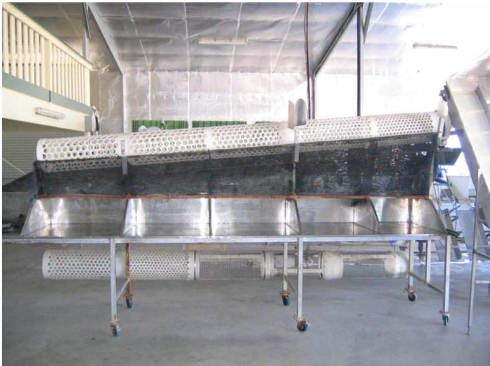
**Figure 2.19:** Rotary grader used for mechanical grading of Pacific oysters (*C. gigas*)
