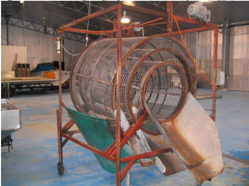
**Figure 2.21:** The Inside/Out grader used for mechanical grading of Pacific oysters (*C. gigas*)
