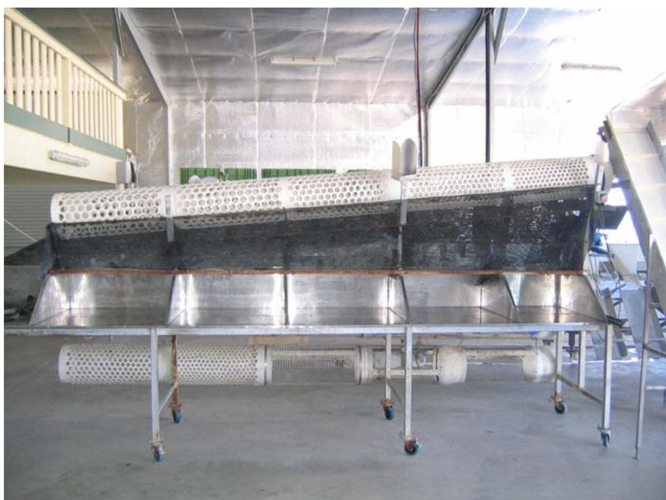
**Fig. A10.2.** The Rotary grader used in this study.
