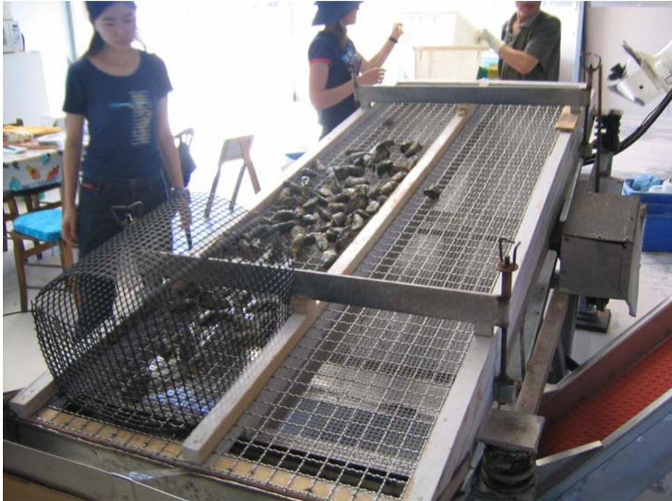
**Figure 2.24.** Mechanical grading of post harvest Pacific oysters (*C. gigas*) using the Flat Bed Grader
