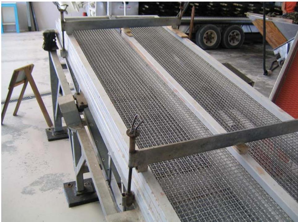
**Figure 2.23.** Flat Bed Grader used for mechanical grading of Pacific oysters (*C. gigas*)
