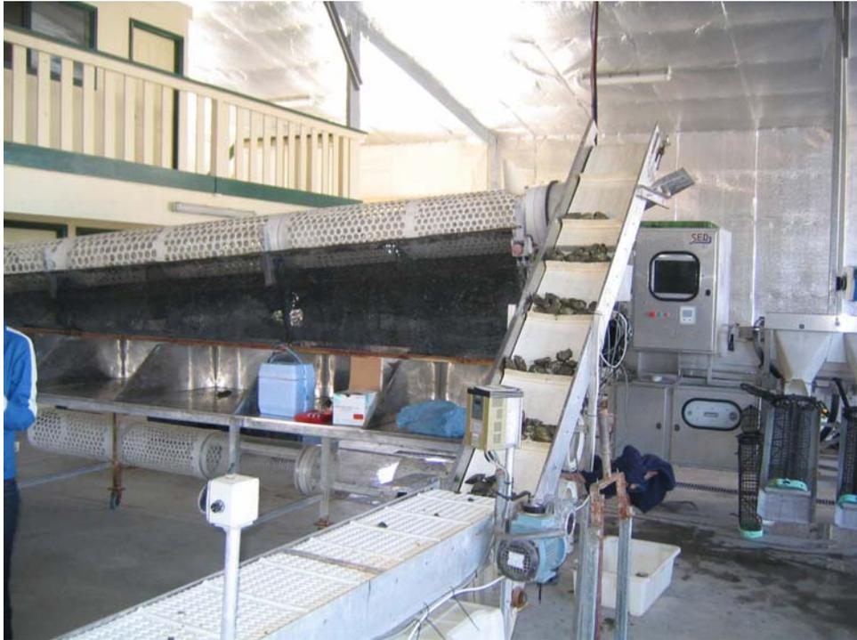
**Figure 2.20:** Mechanical grading of post harvest Pacific oysters (*C. gigas*) using the Rotary Grader
