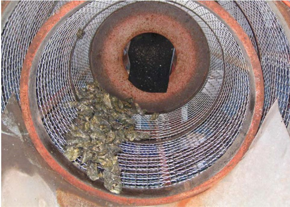
**Figure 2.22.** Mechanical grading of post harvest Pacific oysters (*C. gigas*) using the Inside/Out Grader
