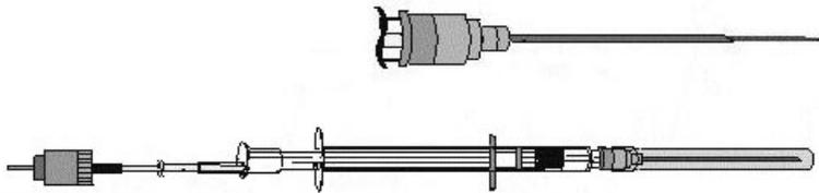
**Fig 3.7 The OxyMicro Systems micro flow fiber-optic oxygen sensor**
