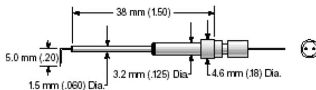
Clark-type oxygen electrodes are the most widely used oxygen sensors. These sensors are based on the reduction of oxygen at a working electrode and are dependant on the diffusion
