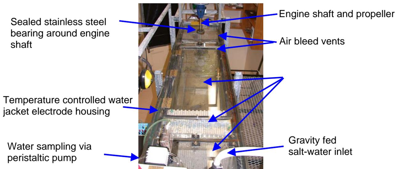
In December 2003 the respirometer was calibrated with respect to flow hydrodynamics and oxygen-holding capabilities. Methods required to measure metabolic rates of YTK were developed in January 2004. The respirometer was used to record the metabolic rates of YTK between 950 and 4350 g with respect to swimming velocity and size. These data allowed calculation of the mass-scaling coefficient for YTK at summer sea water temperatures (22°C).
