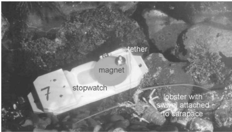
Fig. 1 Juvenile lobster ( Jasus edwardsii ) tethered to a chronographic tethering device (CTD). Lobsters were placed near suitable dens into which they could withdraw for protection.
