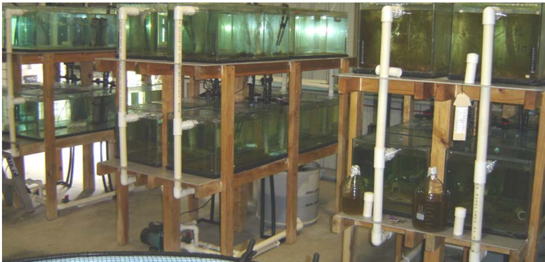
Figure 2.2.2: The recirculation system at the FHU, each bank consisting of eight aquariums, a filter, water pump and an aeration system.
