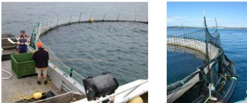
Fig. 6.2. Examples of a typical design used for tuna cages (left – single pontoon with stainless steel ‘seal fence’ above water) and for mulloway or kingfish cages (right – double pontoon with plastic upright structures). Both examples represent the current designs used by each industry. (Photos: D Hamer).
