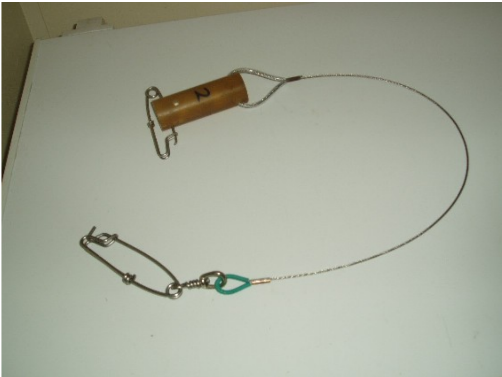
Figure 5. Photo of rigged TDR in protective sheaf.
