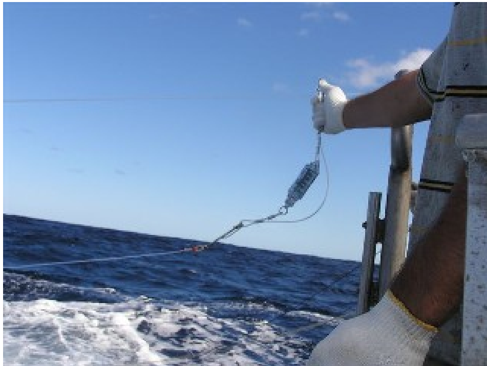
Figure 1. Deployment of rigged hook-timer and branchline.
