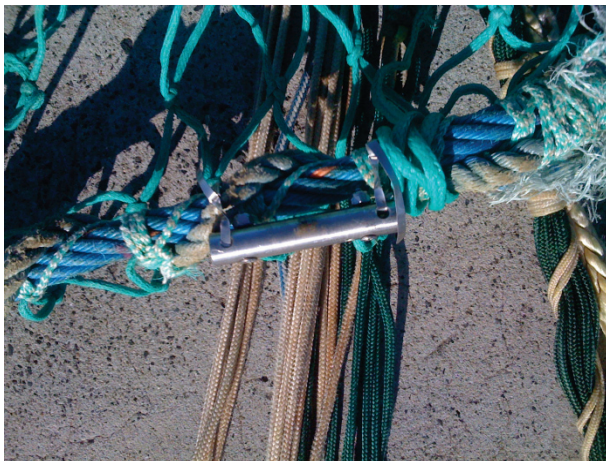
Figure 81. The tag and stainless steel housing attached to the headline of a trawl net. These were further lashed with net twine for security, and the loose ends taped to reduce the chance of entanglement in the net.
