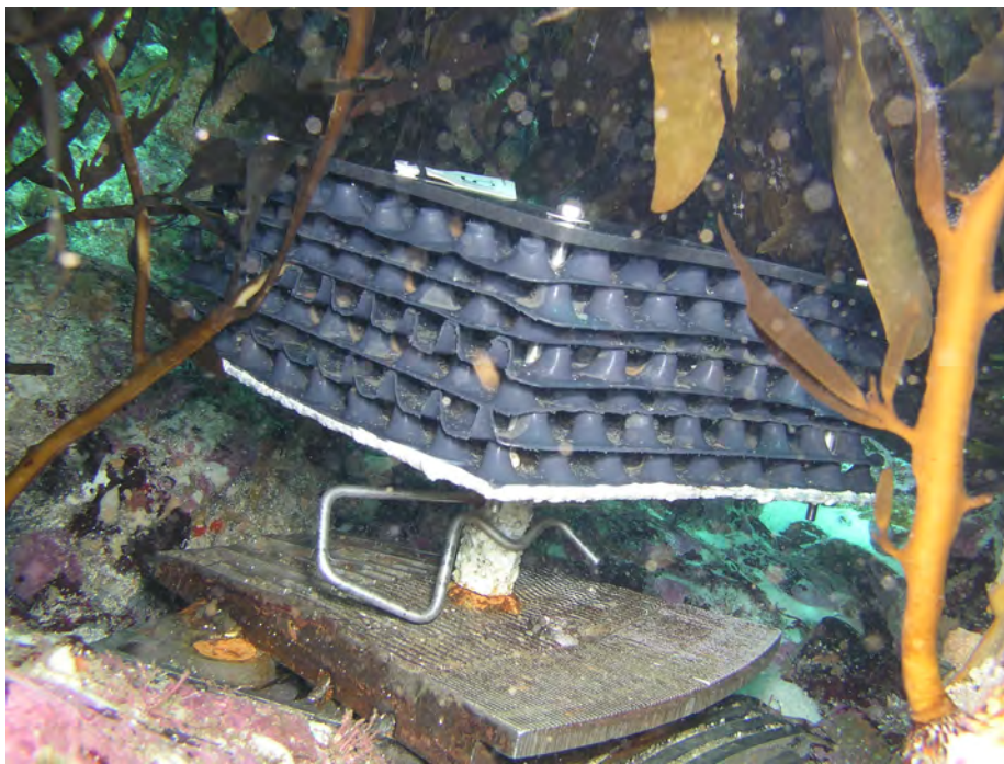
Figure 24. Image of larval collector (Type I) in situ at Pebbly Beach Translocation site. Note the short stipe length of Phyllospora comosa at this site. The head of the collector was designed to sit below the kelp canopy at all sites, to maximise the possibility of intercepting larvae retained below the canopy.
