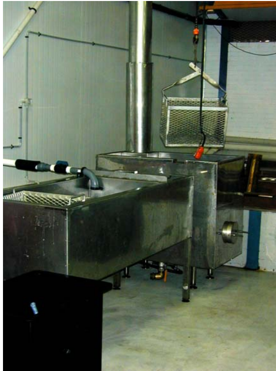
Figure 1: Pilot boiler and ice slurry bath
