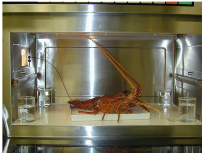
Figure 5: Lobster fitted with fibre-optic probes inside the microwave oven prior to cooking
