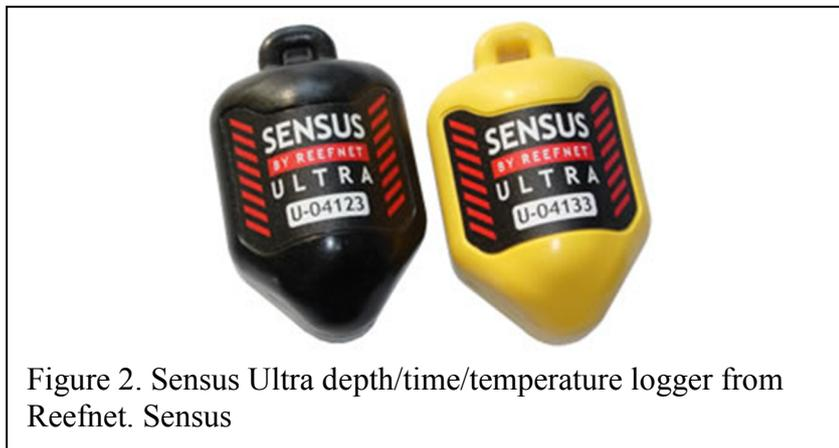
Figure 2. Sensus Ultra depth/time/temperature logger from Reefnet. Sensus
