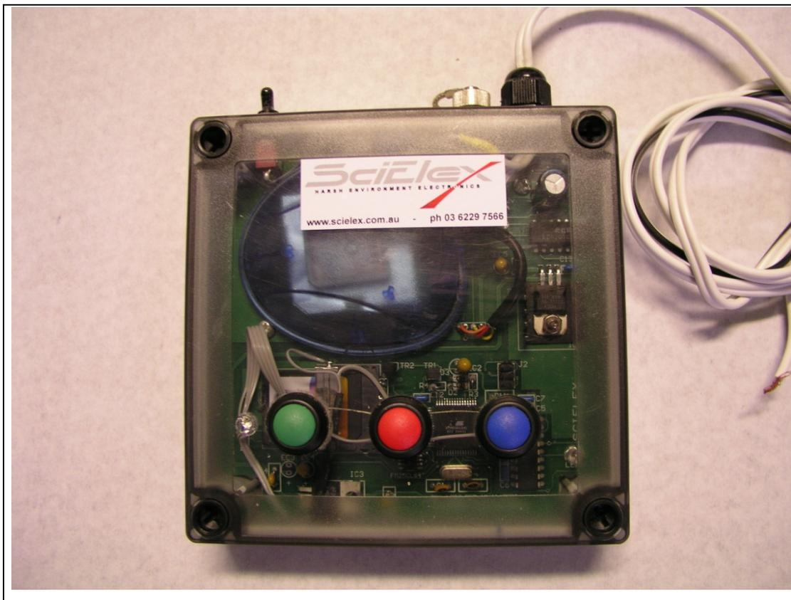
Figure 1. A MKI GPS datalogger with Haicom Hi-204S GPS receiver and external 12v power supply.
