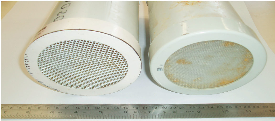
Figure 2. Baitsavers with NITEX mesh sizes of 0.5 mm (left) and 0.05mm (right).
