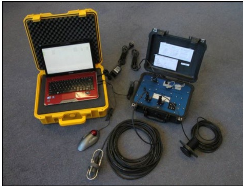
Figure 14. Components of the ARC surface station: laptop computer with ARC control software (left), surface transmitter module (right), multi-directional transducer (bottom centre) and through-hull transducer (bottom right).
