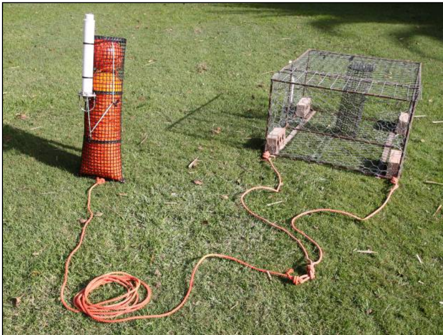
Figure 16. Integration of the ARC-1XDf release unit with a lobster trap.
