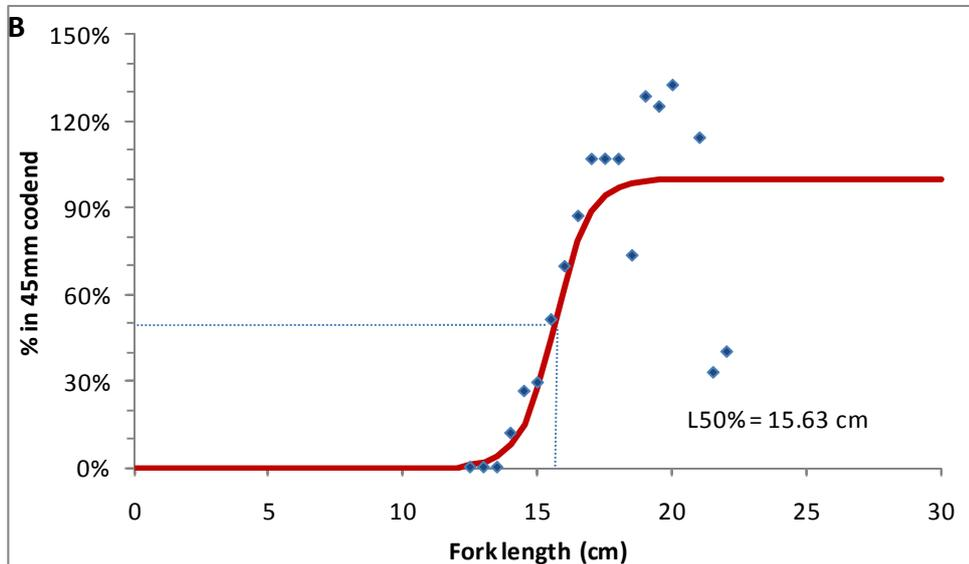
Figure 34. A. Length frequency distribution of Eastern School Whiting that were retained in the 45 mm and 25 mm Eastern School Whiting codends. B. Selectivity of the 45 mm Eastern School Whiting codend for Eastern School Whiting. Each point (♦) marks the % retained at a given 0.5 cm length class and the line (—) represents the estimated logistic selectivity curve.
