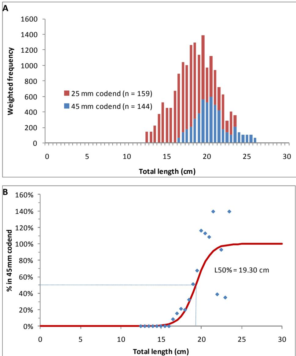
Figure 38. A. Length frequency distribution of Common Stinkfish that were retained in the 45 mm and 25 mm Eastern School Whiting codends. B. Selectivity of the 45 mm Eastern School Whiting codend for Common Stinkfish. Each point (♦) marks the % retained at a given 0.5 cm length class and the line (—) represents the estimated logistic selectivity curve.
