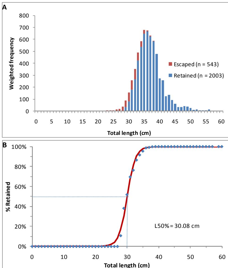
Figure 17. A. Length frequency distribution of Tiger Flathead that were retained in the 75 mm Tiger Flathead codend and those that escaped into the 45 mm codend cover. B. Selectivity of the 75 mm Tiger Flathead codend for Tiger Flathead. Each point (♦) marks the % retained at a given 1 cm length class and the line (—) represents the estimated logistic selectivity curve.
