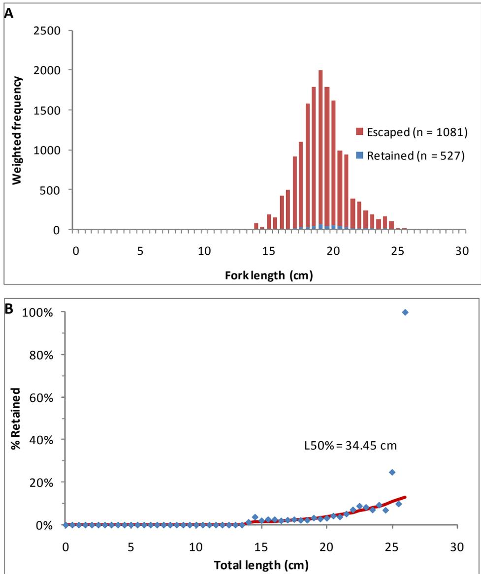
Figure 24. A. Length frequency distribution of Eastern School Whiting that were retained in the 75 mm Tiger Flathead codend and those that escaped into the 45 mm codend cover. B. Selectivity of the 75 mm Tiger Flathead codend for Eastern School Whiting. Each point (◆) marks the % retained at a given 0.5 cm length class and the line (—) represents the estimated logistic selectivity curve.
