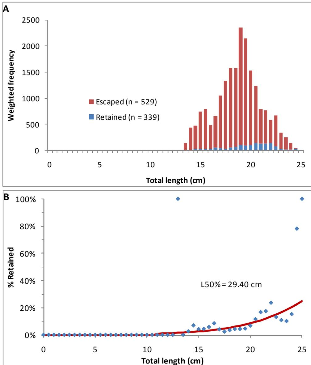
Figure 20. A. Length frequency distribution of Blacktip Cucumberfish that were retained in the 75 mm Tiger Flathead codend and those that escaped into the 45 mm codend cover. B. Selectivity of the 75 mm Tiger Flathead codend for blacktip cucumberfish. Each point (♦) marks the % retained at a given 0.5 cm length class and the line (—) represents the estimated logistic selectivity curve.
