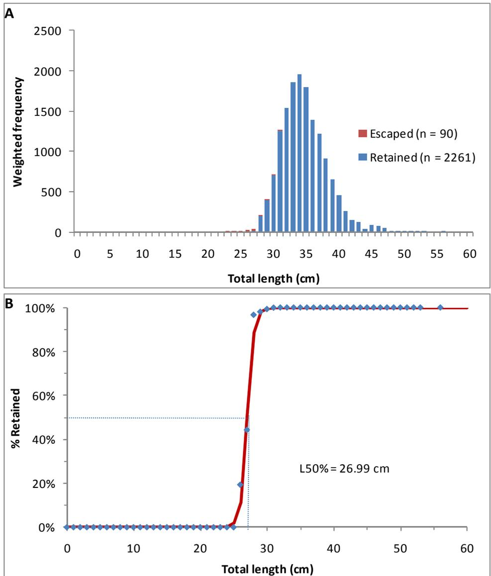
Figure 19. A. Length frequency distribution of Tiger Flathead that were retained in the 65 mm Tiger Flathead codend and those that escaped into the 45 mm codend cover. B. Selectivity of the 65 mm Tiger Flathead codend for Tiger Flathead. Each point (♦) marks the % retained at a given 1 cm length class and the line (—) represents the estimated logistic selectivity curve.
