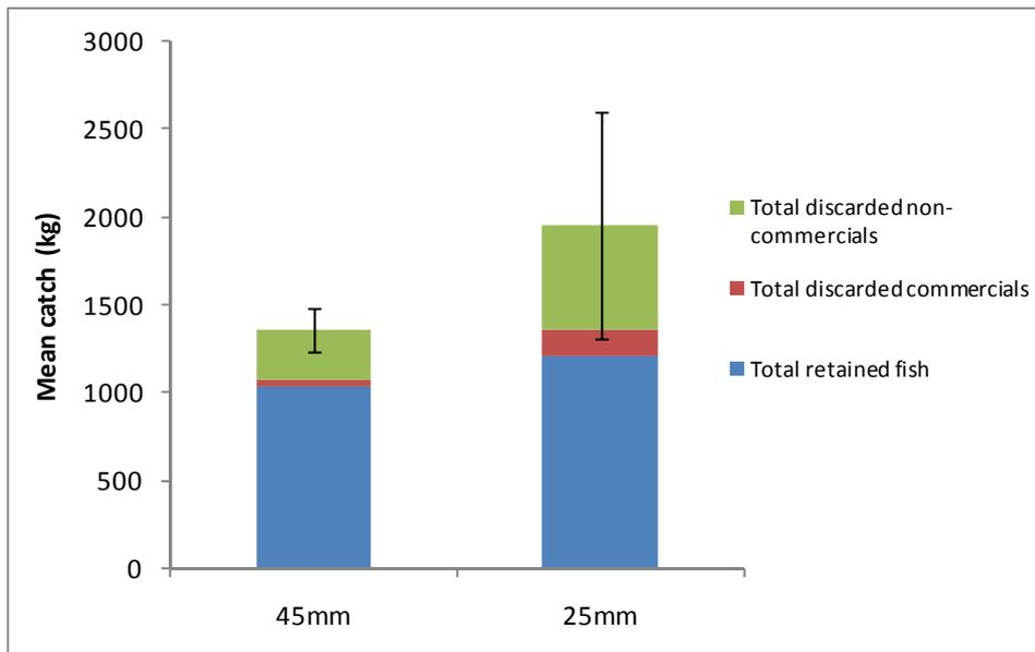
Figure 29. Mean total catch rates (+ SE) by the 45 mm and 25 mm codends.
