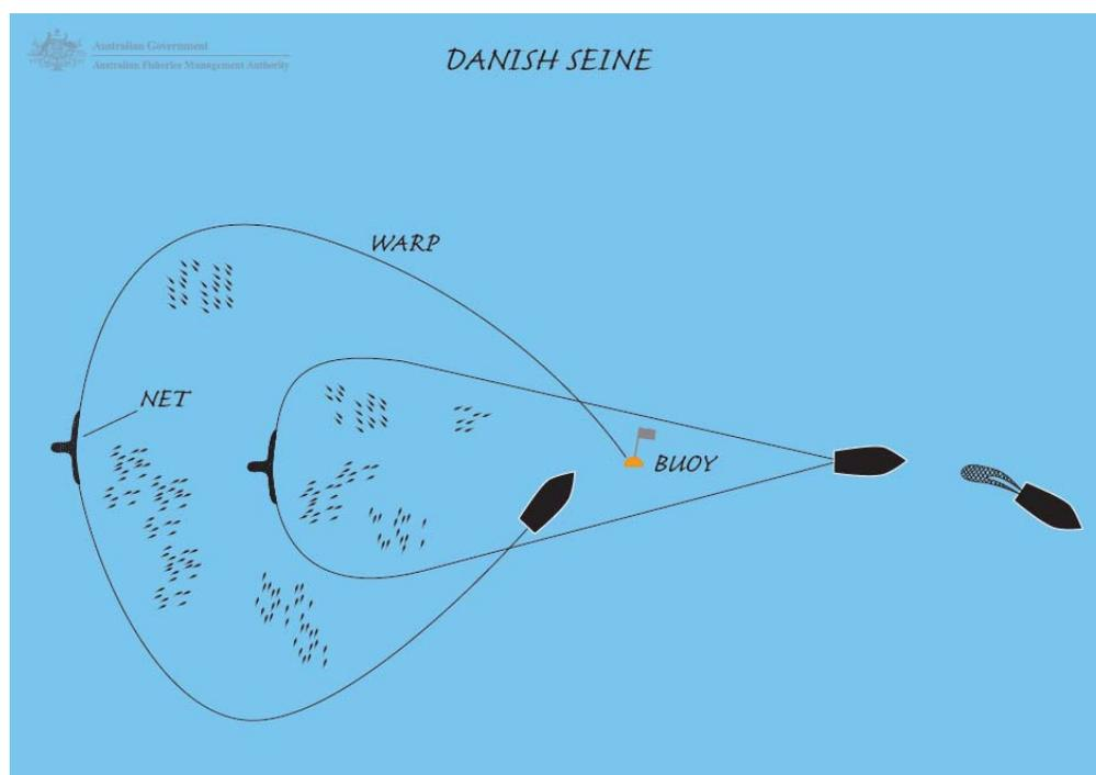
Figure 41. Operation of Danish seine gear from when the net is set to just before hauling. Reproduced from Australian Fisheries Management Authority website (<http://www.afma.gov.au>).
