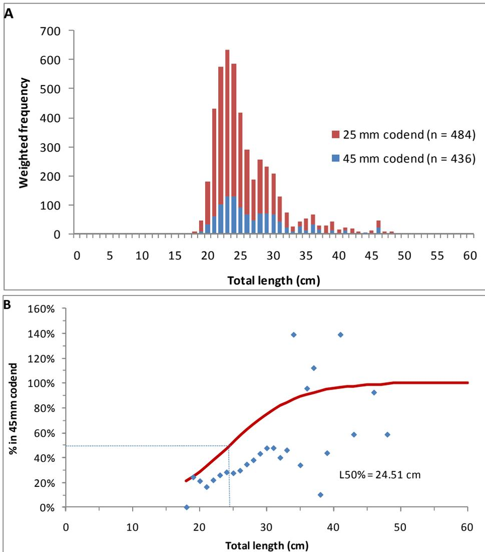
Figure 36. A. Length frequency distribution of Tiger Flathead that were retained in the 45 mm and 25 mm Eastern School Whiting codends. B. Selectivity of the 45 mm Eastern School Whiting codend for Tiger Flathead. Each point (◆) marks the % retained at a given 0.5 cm length class and the line (—) represents the estimated logistic selectivity curve.
