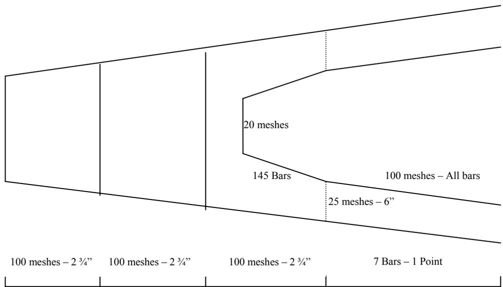
**Figure 1. Net design that was used throughout the project. Different codends were attached for different experiments.**
