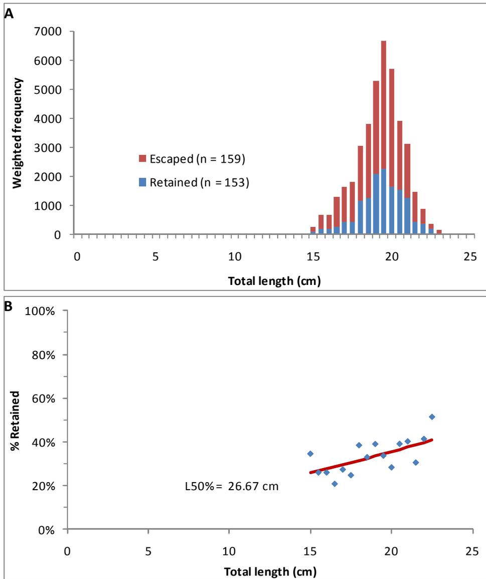
Figure 22. A. Length frequency distribution of Blacktip Cucumberfish that were retained in the 65 mm Tiger Flathead codend and those that escaped into the 45 mm codend cover. B. Selectivity of the 65 mm Tiger Flathead codend for blacktip cucumberfish. Each point (♦) marks the % retained at a given 0.5 cm length class and the line (—) represents the estimated logistic selectivity curve.
