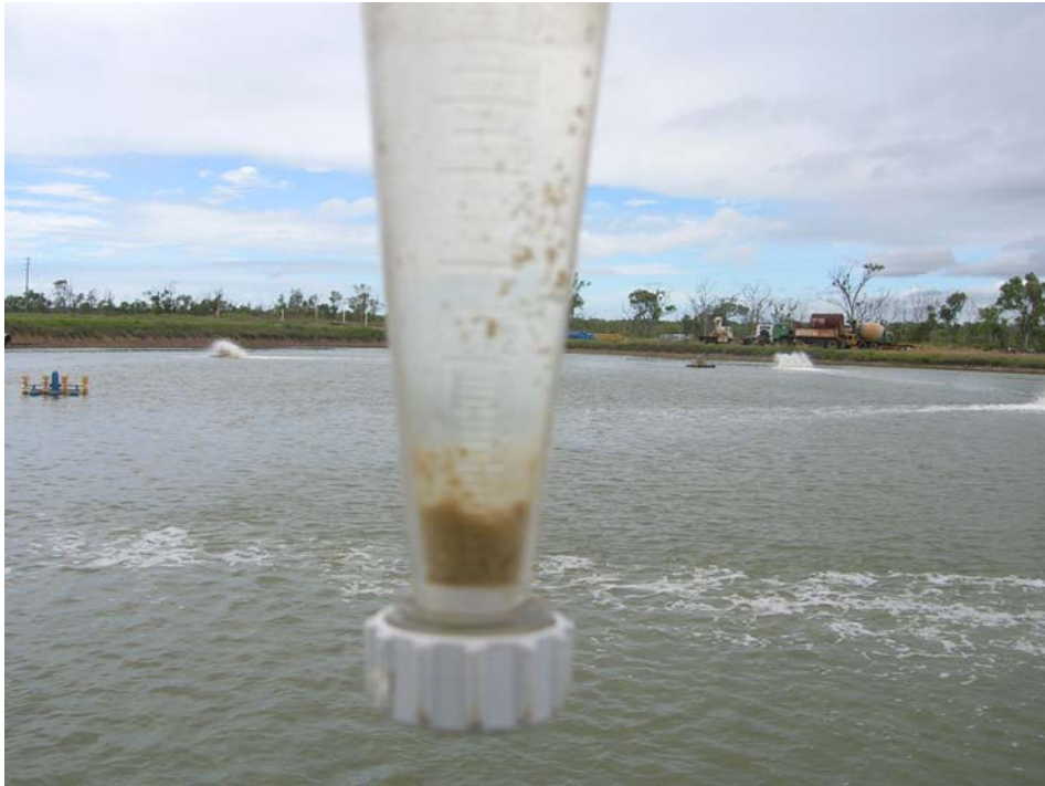
Photograph 3. Biofloc (~ 0.5 mL) settling out in an Imhoff cone.
