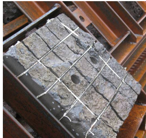
Ceramic and oyster shell aggregate algal settlement panels Cheju Do, Korea
