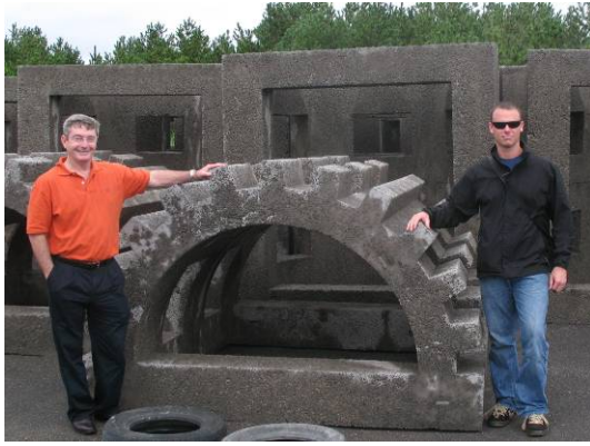
Oyster shell aggregate module for algae and top shell Cheju Do, Korea
