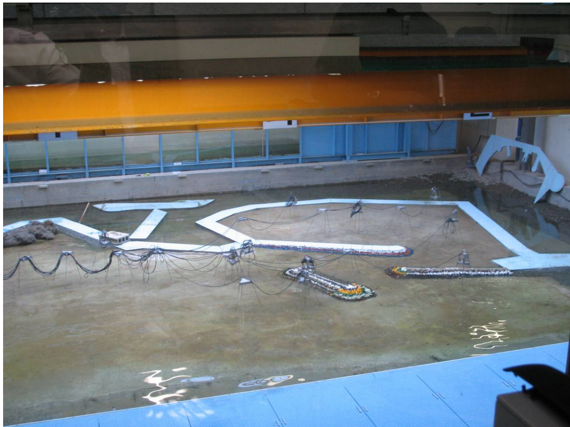
Hydraulic testing for reefs and breakwaters, Japan
