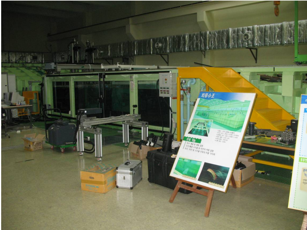
Flume tank for testing artificial reefs, Busan Korea
