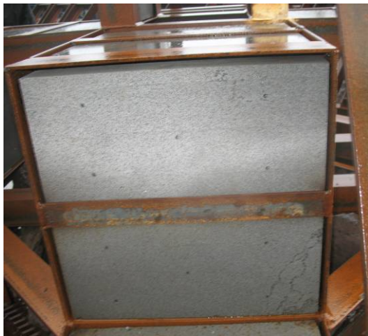
Ceramic and oyster shell aggregate algal settlement panels Cheju Do, Korea
