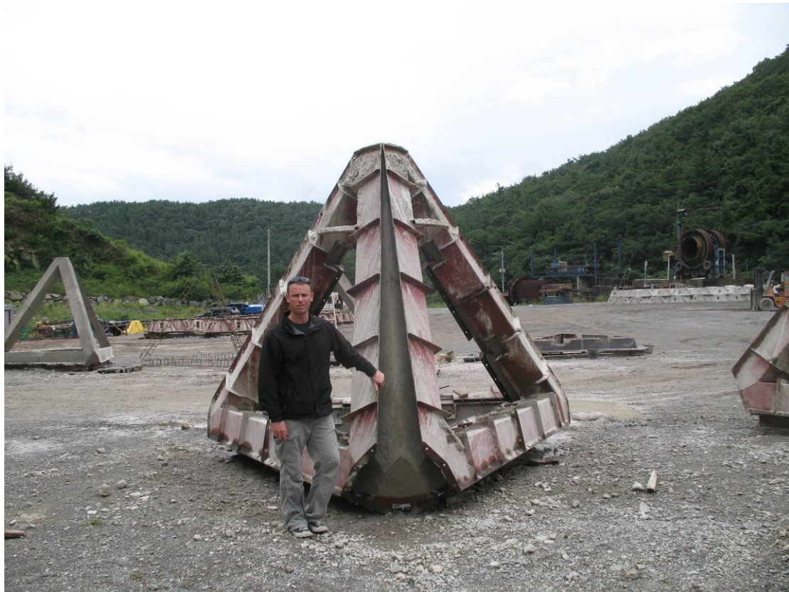
Mixed purpose reef construction, Korea
