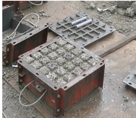
Algae and shellfish concrete reef modules and oyster shell attachment plate Cheju Do, Korea
