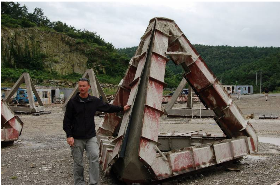
Concrete reef moulds, Korea
