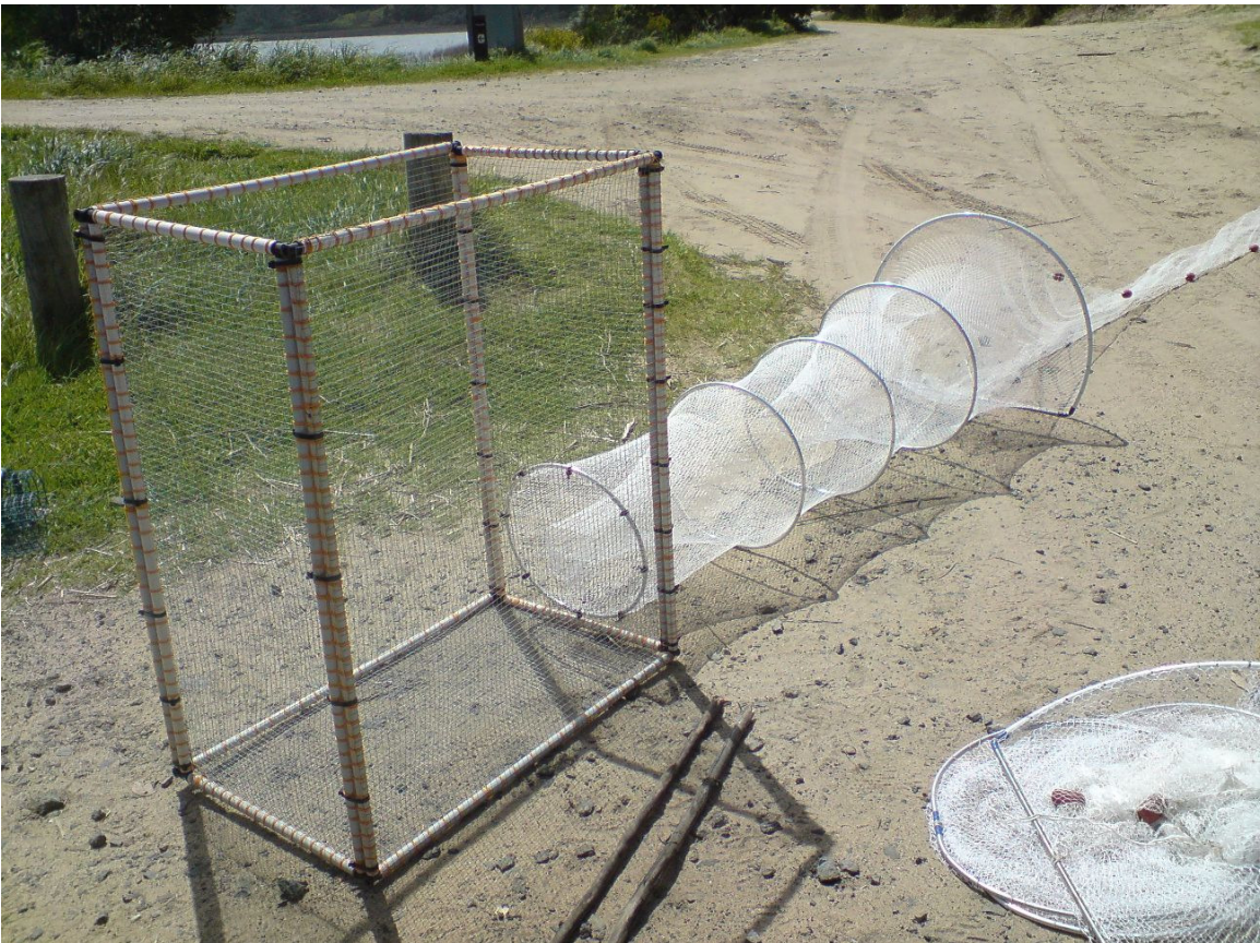
Figure 3. Modified fyke net with rigid frame cod end.
