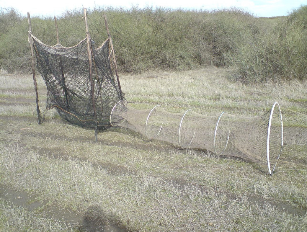
Figure 4. Modified fyke net with collapsible cod end.
