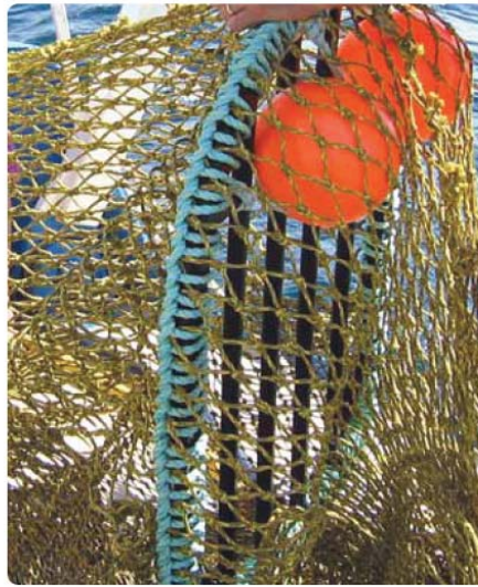
Figure 16. Floats attached inside the net must be behind the grid
