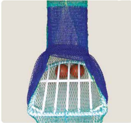
Figure 7a. Single flap, triangle escape hole opening. The TED is attached to the circumference of the net with heavy twine
