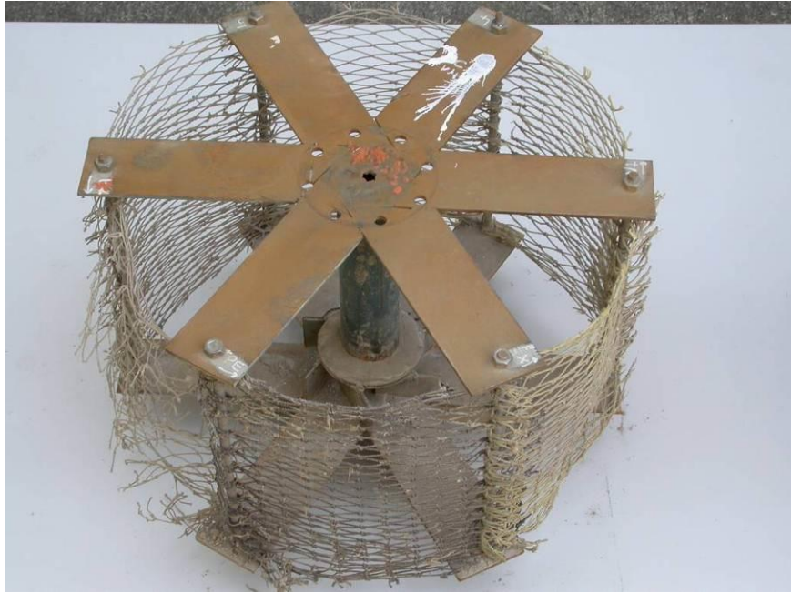
Figure 18: Wear-application wheel and mounted netting pieces after the wear treatment was applied.
