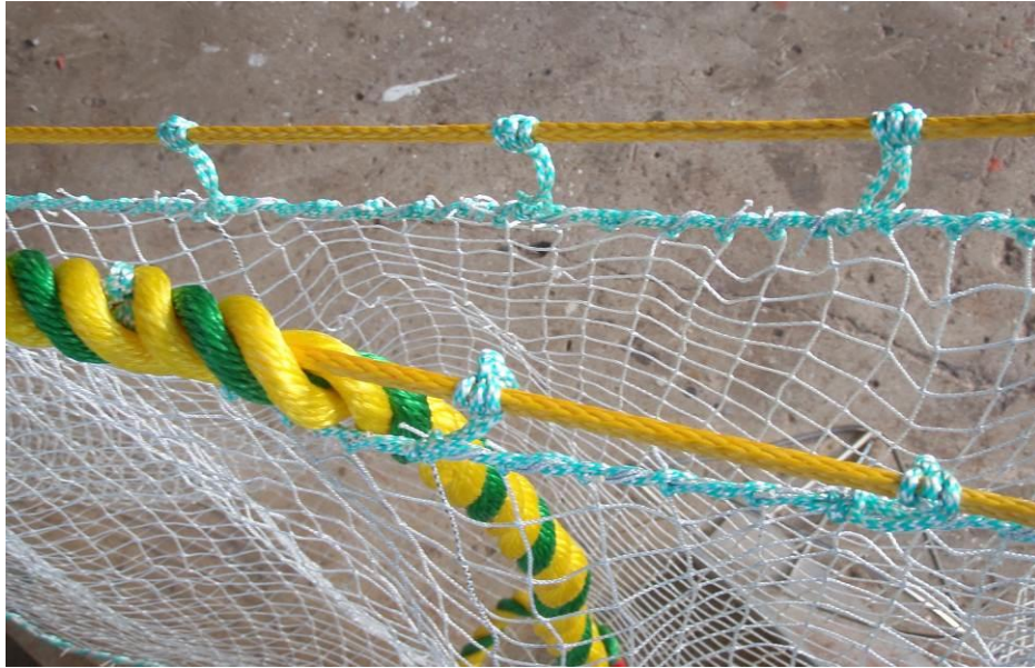
Figure 47: Dyneema frameline configuration for the Ultracross trawl – The fishing line was wrapped with 20mm PE.
