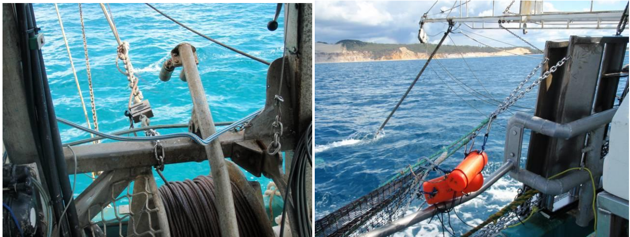
Figure 51: Load and spread measuring instrumentation attached to the trawl gear.
