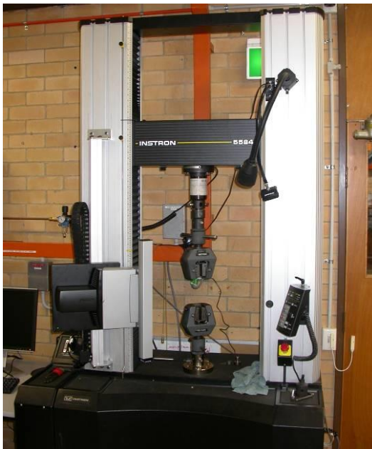
Figure 4: Pictures of the utilised Instron tensile testing machine and a polyethylene netting sample loaded for testing in the machine.
