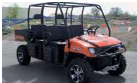
Larger small vehicle fitted with a rollover protection structure (ROPS)
