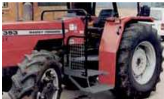
The same tractor fitted with a safe access system.
