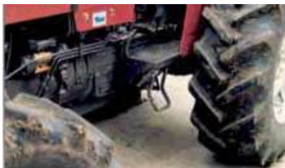
Access is from in front of the rear wheels. A safe access platform is necessary to reduce the run-over hazard.
