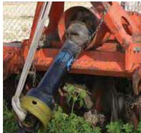
The red circular metal guard covers the universal coupling joining the PTO shaft to the implement. The restraining chain and tie are used to stop the PTO shaft from falling onto the implement
