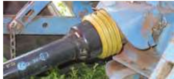
Clip-held removable Master Guard covering the connection of PTO shaft to tractor PTO
