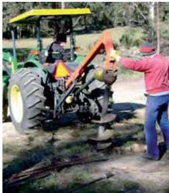
The worker standing behind the digger is in danger of being struck and/or entangled if the auger hits an object and jumps from the hole. Wire, steel posts and tools lying near the posthole increase the hazard
