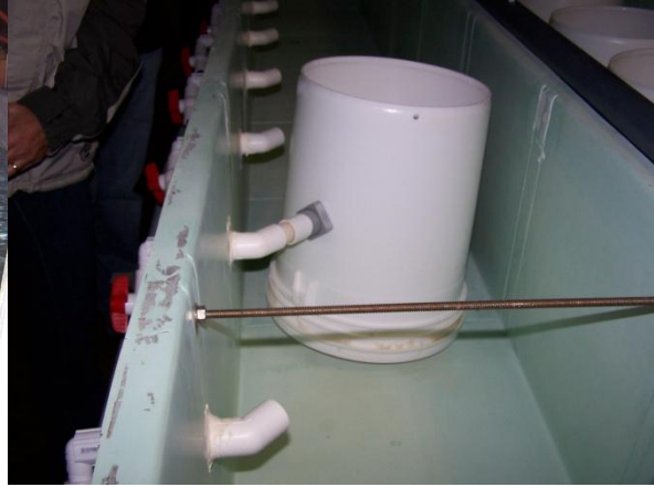
Upweller with 'ice cream bucket' screen
