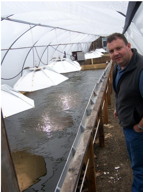
Three meter deep algae tanks
