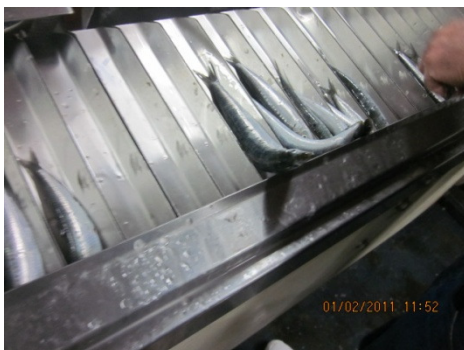
Figure 16: Feeding conveyor issues (inefficient use of fish slots)
