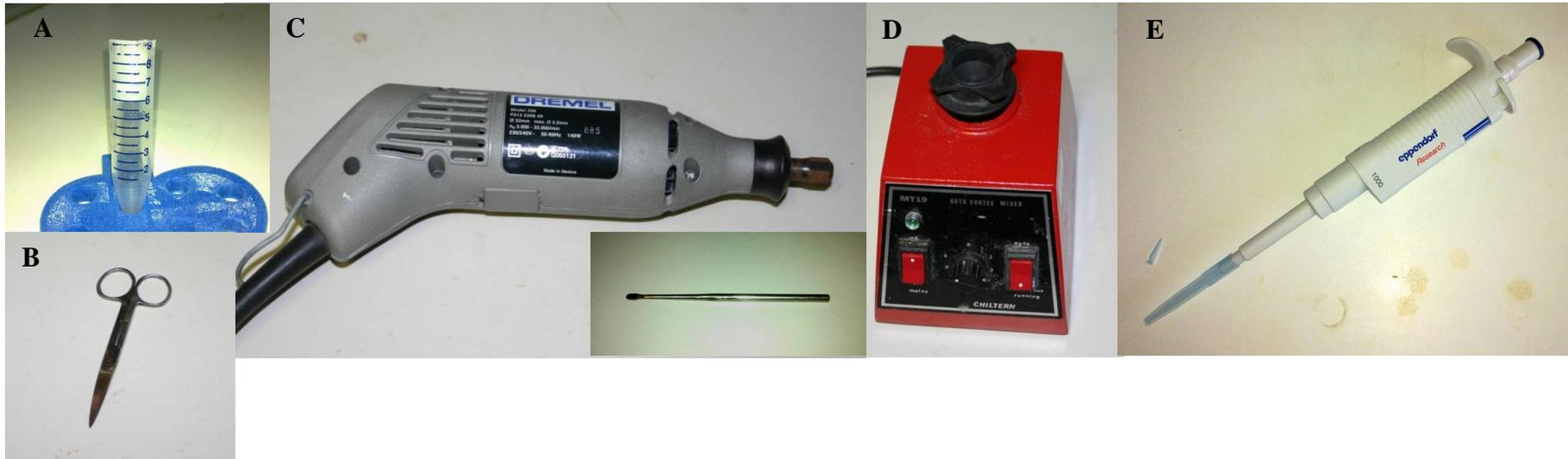
**Figure 13.** Equipment used in the preparation of sperm suspensions for estimating sperm number and morphology. A. Tube cut to a depth to allow fine point scissors to reach the bottom. B. Fine point scissors. C. Dremel drill and custom made cutting tool (inset). D. Vortex. E. 1mL pipette and tip with end removed.
