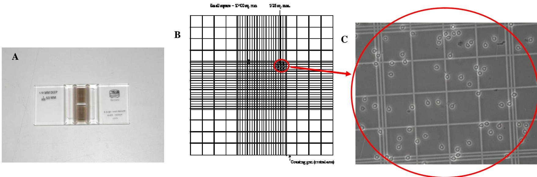
**Figure 14.** A. Haemocytometer. B. The grid of a haemocytometer is divided into 9 large squares with each square having a surface area of 1 square mm and the depth of the chamber is 0.1 mm. Prawn sperm cells are counted using the 1/25sq.mm grid squares. C. Sperm cells within a 1/25sq.mm grid, which is made up of 16 smaller 1/400sq.mm squares.
