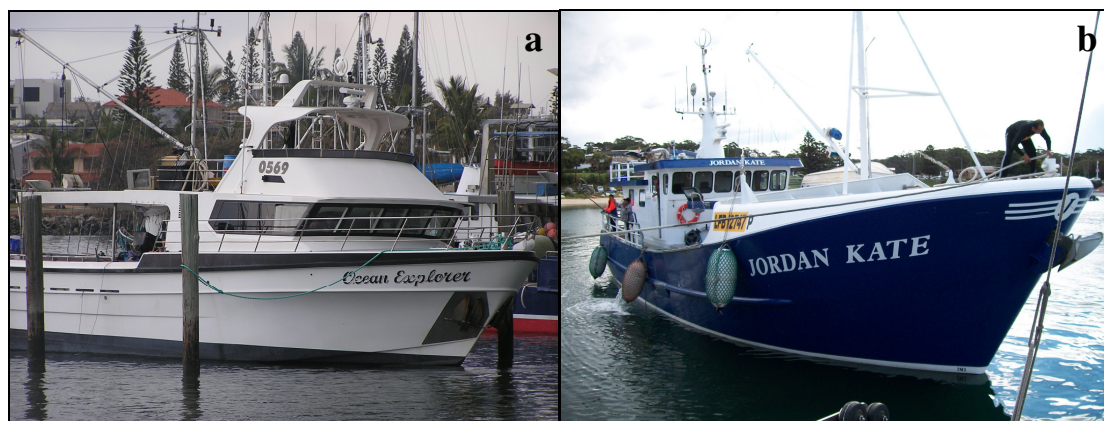
Figure 2: Variations in trial vessel designs include (a) forward wheelhouse fibreglass FV Ocean Explorer and (b) aft wheelhouse steel FV Jordan Kate .
