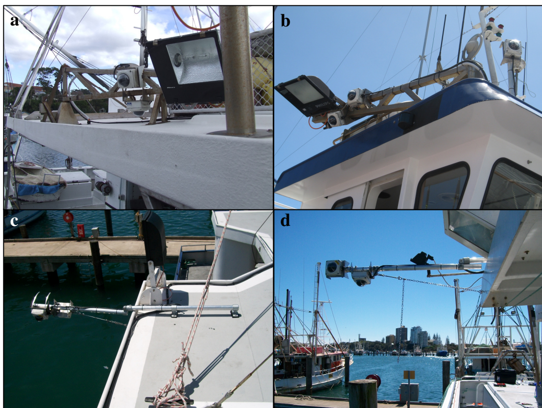
Figure 6: Cameras placed to enable an outboard view of fishing gear retrieval and catch handling on vessels existing boom (a) FV Bianca B , (b) FV Jordan Kate , and fabricated and installed boom (c) FV Beluga and (d) FV Ocean Explorer .
