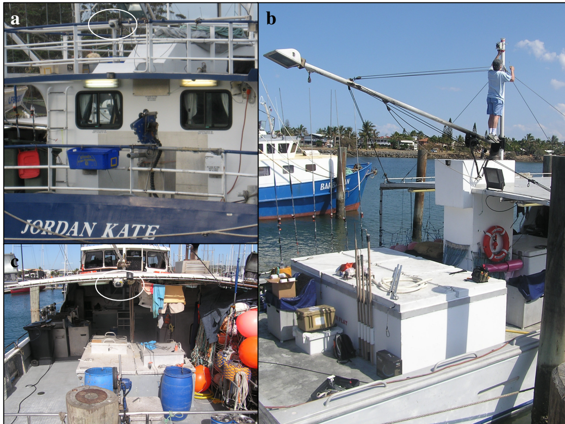
Figure 7: Cameras placed to capture views of fishing gear deployment on project vessels (a) FV Jordan Kate , (b) FV Blue Mistress , and (c) FV Samurai .
