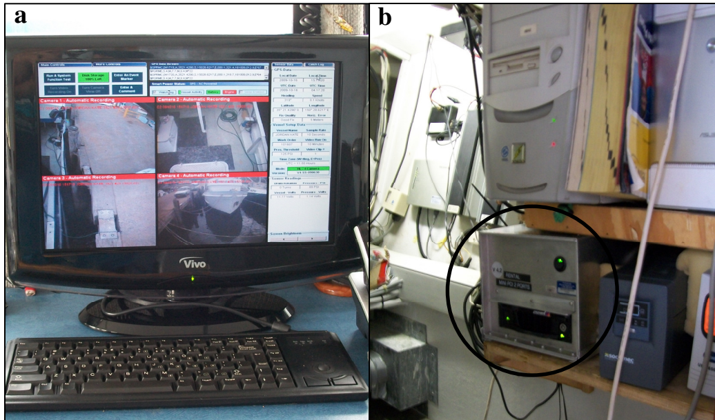
Figure 9: System monitor (a) and circled control centre (b) installed on project vessels.
