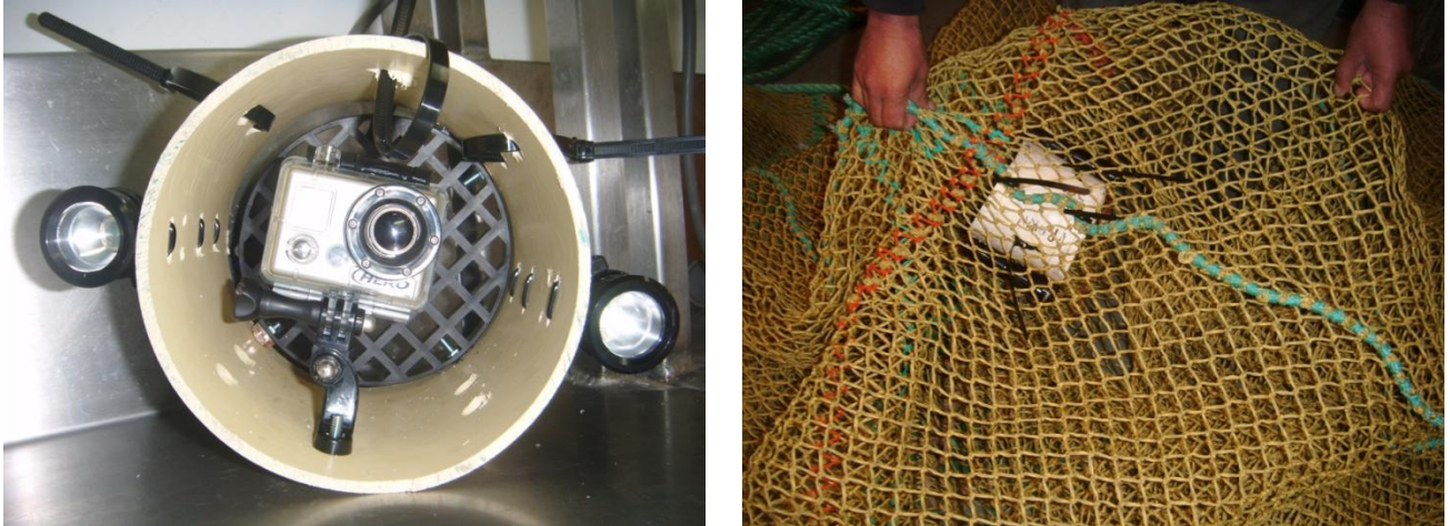
Figure 2. Hero® HD digital video camera and mount (including lights) (Left) and attached to the inside of the cod-end (Right).
