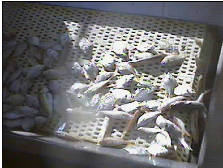
Figure 20: Glare impacting image quality during early morning on the conveyor.
