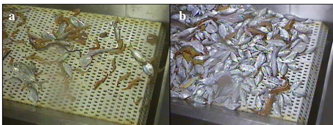
Figure 11: Camera view at the end of the conveyor showing (a) small non-commercial prawns being directed to the discard chute and (b) clearly observed tiger prawns amongst fish bycatch.
