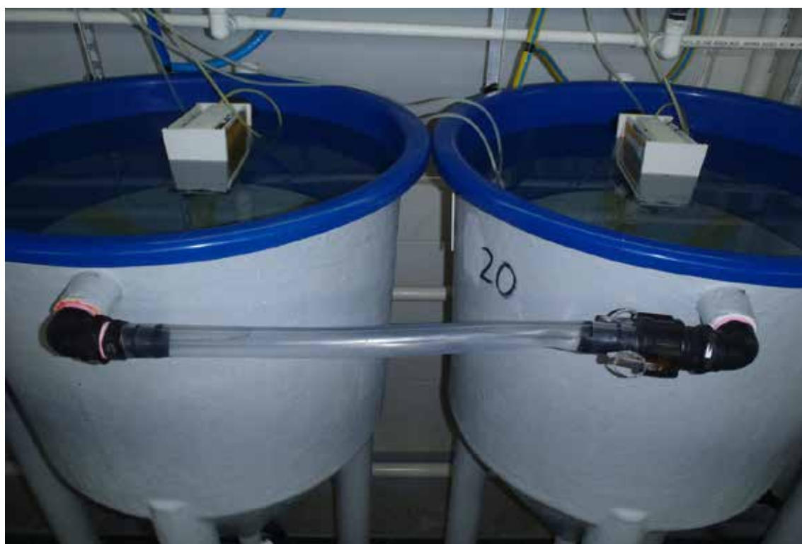
Figure 6. A pair of 270 Lt tanks connected during larvae transfer
