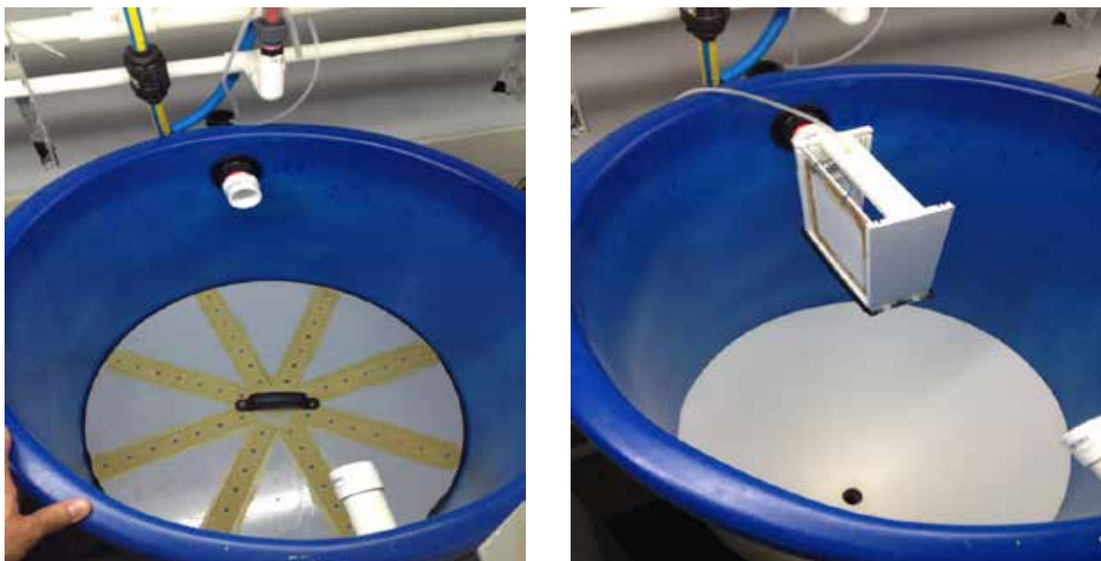
Figure 5. 270 Lt tank containing the false bottom (left) box filter with interchangeable screens (right).
