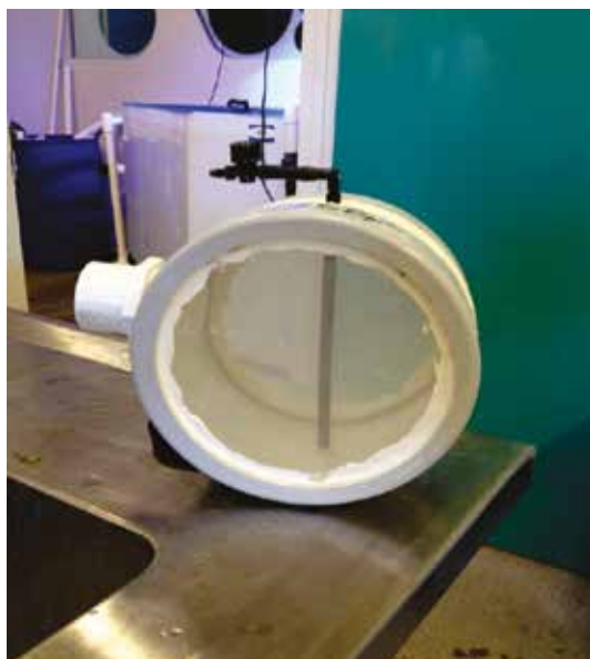
Figure 2. Banjo screen profile (left) and its locality in the 40 L tank, green arrow indicating poly valve and riser (right).
