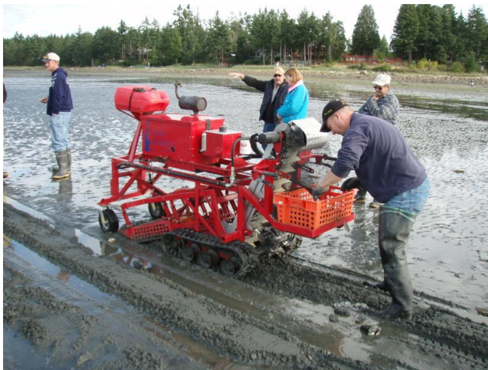
Figure A8. A mechanical clam harvester used on the west coast of the USA.
