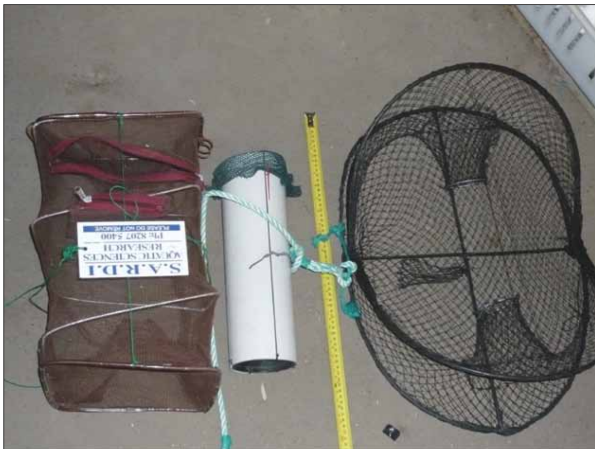
Figure 3. Three trap types used by SARDI. From left to right: box, pipe and opera house traps.
