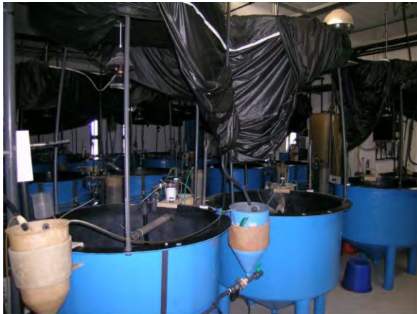
Intensive larval rearing replicated system
