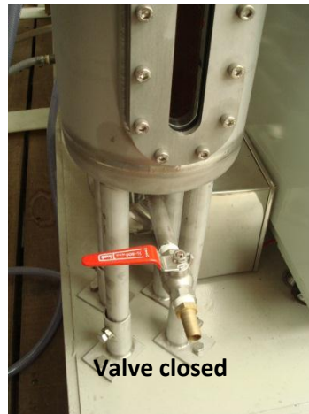
Figure 15. Water reclaim valve on the bottom of the pot. Used for collecting the reclaimed water from the drying process
