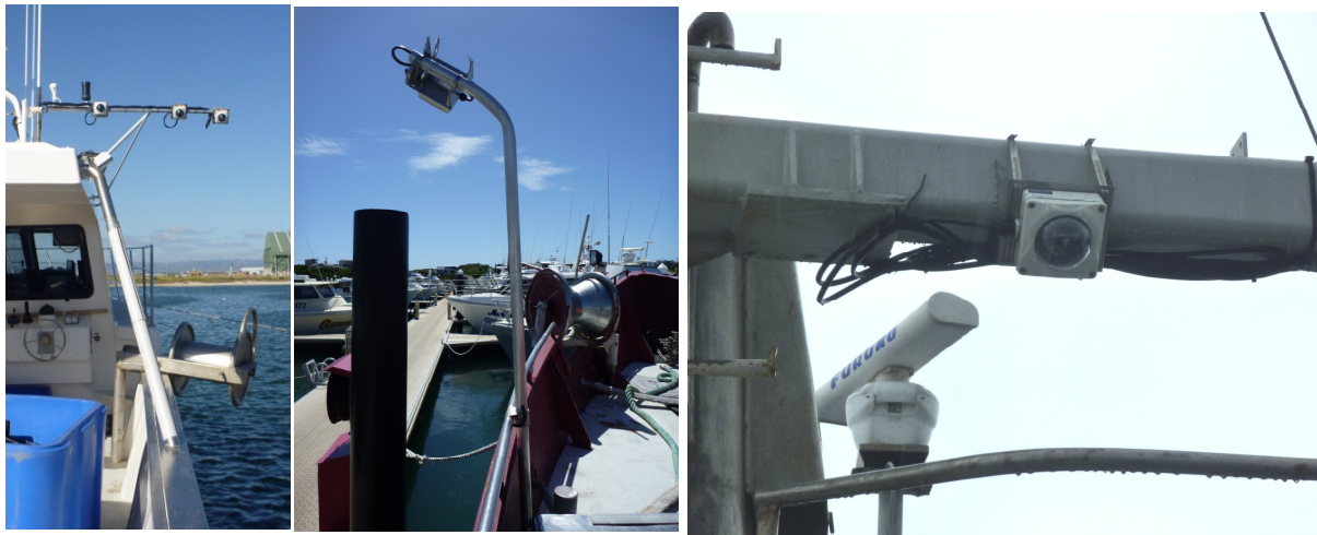
Figure 4: Closed circuit television cameras mounted on Commonwealth fishing boats as part of electronic monitoring systems
