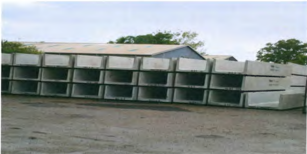
Concrete culverts destined for the Lee Point artificial reef complex near Darwin
