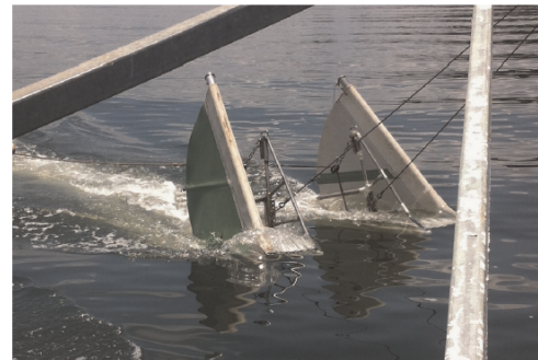
Fig. 2. Second commercial prototype (CP2) batwing otter board being deployed in the field (McHugh et al., 2015).
